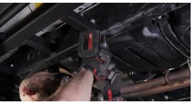
**6.** Use a 1/2" bolt with a washer and a flange nut to secure the slider to the drilled bolt holes.
