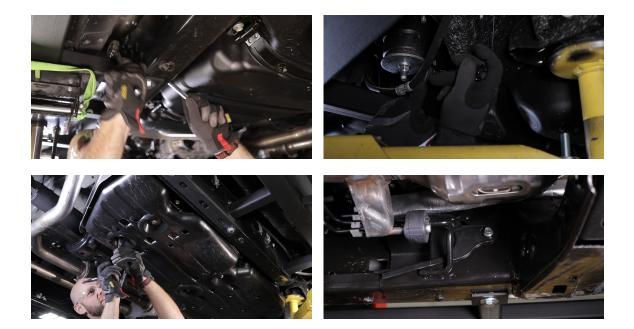
On the passenger side you will repeat the same steps except you will not have to remove the gas tank cover. There will be brake lines in the way but those can easily be moved by popping them out of their clip. Make sure all bolts are tightened down and you are finished with the install.
