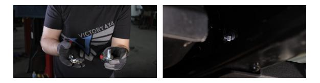
Use a 12mm wrench to remove the bolt holding up the brake line. Use the bracket we provide to secure the bolt next to the gas tank that it difficult to reach.
