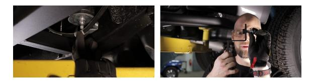
**5.** Begin drilling with a small bit to open a hole, then use a step bit to open the hole to a 1/2". You will be drilling 3 holes in the frame.
