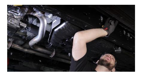
**2.** Remove the 6 bolts holding up the gas tank cover using a 12mm socket. Then remove the plastic cover inside the frame using a 12mm socket.
