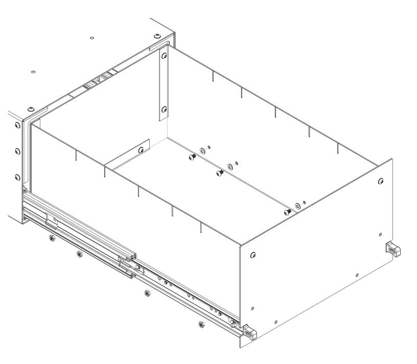
**9.** With your drawer attached to your slides, you can now assemble the handle system around the red latches on the slides. To do so, use (4) of the provided button heads and secure them through the "PRESS" bracket into the pem nut bracket and sandwhich them around the red grab handles so they are grabbing them, as shown in the orientation below. You may need to preload the assembly with a clamp before final torque to ensure proper fitment.
