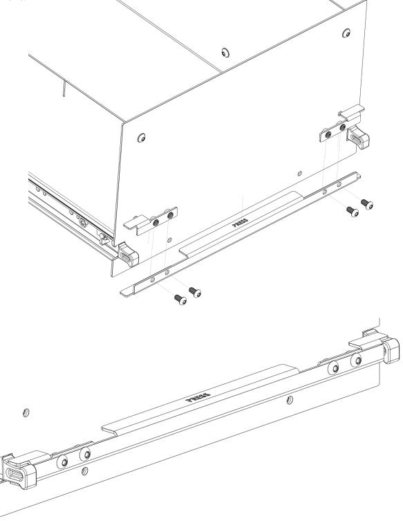
**10.** The final step is to secure the handle cover bracket to the front of the drawer to complete your install. Take (4) of the provided 1/4" button heads, washers and flange nuts and use them to secure the bracket to the panel, as shown in the orientation below. \*If you've purchased our label kit, you will install them here before securing the handle cover.
