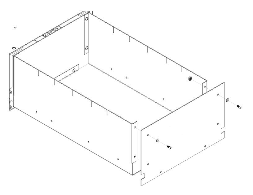
**8.** With the front piece in place, you now need to attatch the drawer assembly to your slide system using (4) of the provided 1/4" x 3/8" long button heads with loctite applied to them, with washers and flat nuts on each side, as shown in the orientation below. Be sure that the button heads are installed from the inside of the drawer facing out. You will need to adjust the length of the slide to access some of the bolt holes.
