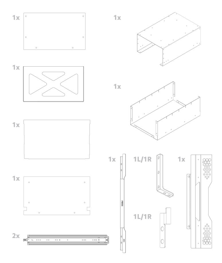
1. Start by taking the (2) provided slides and bolt one to each side of the inside of the slide assembly with the red handles pointing out, as shown in the orientation below. Making sure to use (4) each per side of the provided shorter 1/4" button heads, washers and flat nuts and apply the provided blue loctitie to the bolts before tightening. You will need to extend the slide to access some of the mounting holes on the inside.
