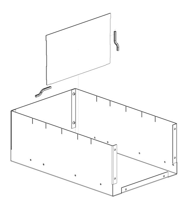
7. You can now start to fasten the front drawer piece onto the drawer assembly. To do so use (2) of the provided 1/4" x 3/8" long button heads, washers and flange nuts, as shown below.
