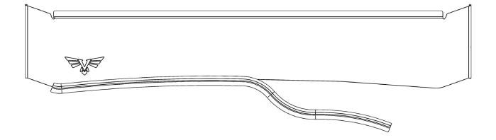
**3** Next, mount the front and rear fairings. To do this, use the 1/4"-20 X 3/4" button head bolts, 1/4" ID washers, and 1/4"-20 serrated flange nuts. The front fairing will need 3 of each per side and the rear fairing will need 2 of each per side. When mounting the front fairing, adjust it all the way up to avoid contact with the roof and leave the bolts loose enough to be able to make adjustments once it is on the roof of the vehicle.
