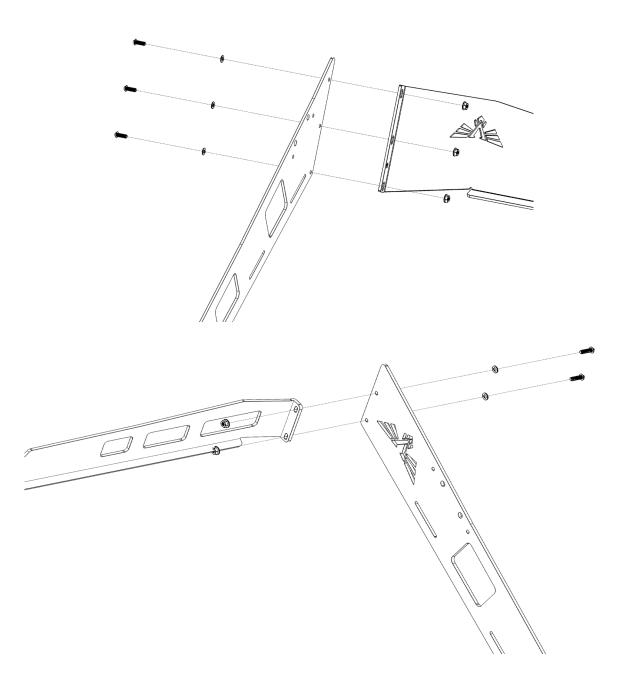
4 Next, attach the 1 and 3 mounts to the assembled roof rack using the 1/4"-20 X 3/4" button head bolts, 1/4" ID washers, 1/4"-20 serrated flange nuts. Insert the 5/16" carriage bolts into the square cutouts in the 3 mounts before installing them. Tighten them fully to the inside of the side rail. Make sure that the arrow is pointing forward. The front mounts should mount to the second set of holes in the side rails.
