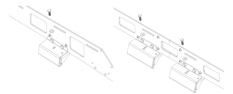
Due to the variance in manufacturing of these van roof panels, some manipulation of these brackets may be required for proper installation. This rack is entirely secured using clamping force, and it relies on tight tolerances in the mounting brackets to ensure it remains safely attached to the vehicle.
