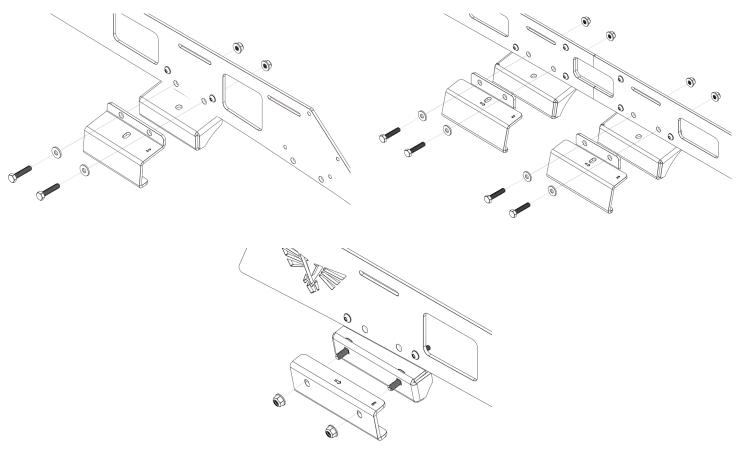
The outer clamps should be drawn into the inner mounts and secured to the drip rail using the (2)  $5/16" \times 1 1/2"$  bolts and nylon locking nuts that pass thru the side rails. If the two mounts are too far separated initially to start the clamping hardware, a C-clamp or F-clamp can be used to pull the mounts together enough to get the hardware started.
