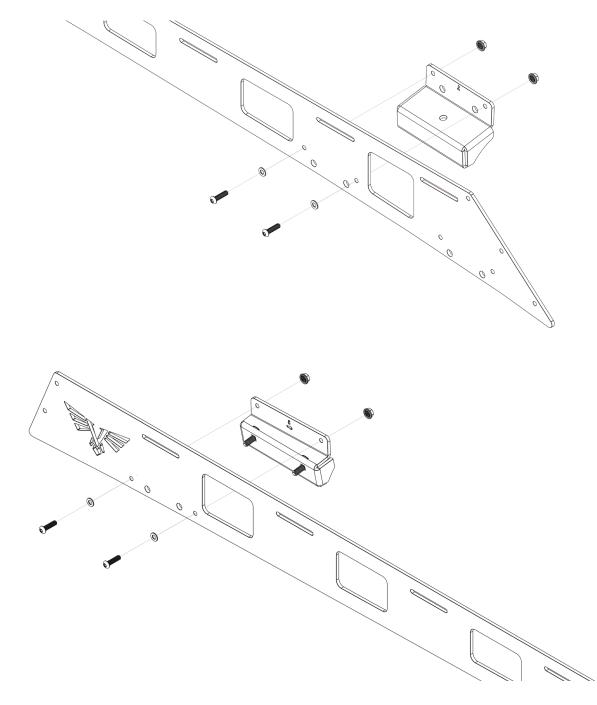
5 Next, place the 2 halves on the roof of the vehicle and attach them using the 1/4"-20 X 3/4" button head bolts, 1/4" ID washers, 1/4"-20 serrated flange nuts and the connecting bracket. Only use the top 2 holes because the other mounting point will be used later on. When placing the rack on the roof, position it so the points on the front fairing sit roughly 2" behind the top edge of the windshield.
