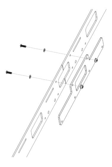
6 Next, lift the rack slightly and attach the mid mounts using the 1/4"-20 X 1" button head bolts, 1/4" ID washers, 1/4"-20 serrated flange nuts. Tighten them fully to the inside of the side rail.
