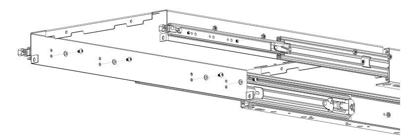
**4.** Once you have your bracket installed to the slides in the orientation of your choice, you can now bolt the back piece to your bracket. To do so use the provided 1/4" button heads, washers and nuts as shown in the orientation below.
