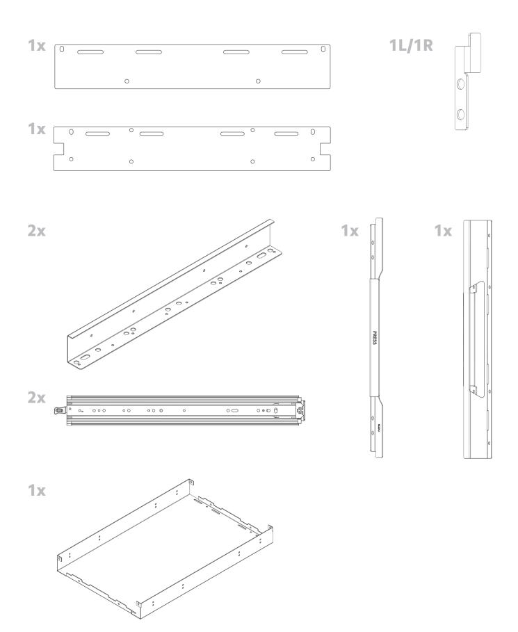
1. Start by taking the (2) provided slides and bolt each one to the insides of the provided floor mounts, making sure the red handles are pointing out, as shown in the orientation below. Make sure to use (4) each per side of the provided shorter 1/4" button heads, washers and flat nuts and apply the provided blue loctitie to the bolts before tightening. You will need to extend the slide to access some of the mounting holes on the inside.
