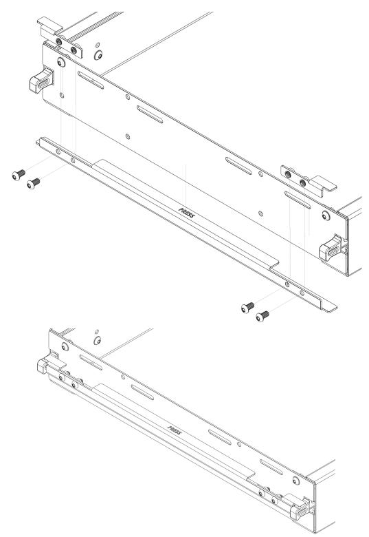
7. Once the handle is assembled, you now need to place the cover over the assembly using (6) each of the provided button heads, washers and flange nuts. This is also the step you need to remove the hardware from step 5 if your tray is facing upright, and then place back over the cover piece. Assemble in the orientation shown below.
