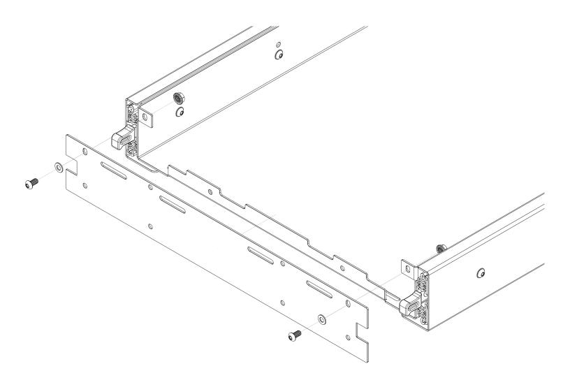
6. You are now ready to assemble the handle system around the red latches on the slides. To do so, use (4) of the provided button heads and secure them through the "PRESS" bracket into the pem nut bracket and sandwhich them around the red grab handles so they are grabbing them, as shown in the orientation below.
