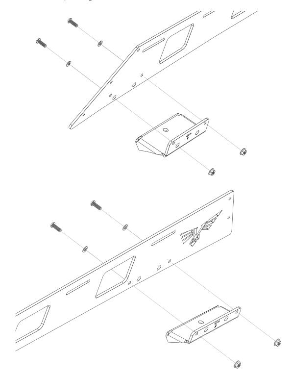
5 Next, place the 2 halves on the roof of the vehicle and attach them using the 1/4"-20 X 3/4" button head bolts, 1/4" ID washers, 1/4"-20 serrated flange nuts and the connecting bracket. Only use the top 2 holes because the other mounting point will be used later on. When placing the rack on the roof, make sure it is positioned behind the antenna.
