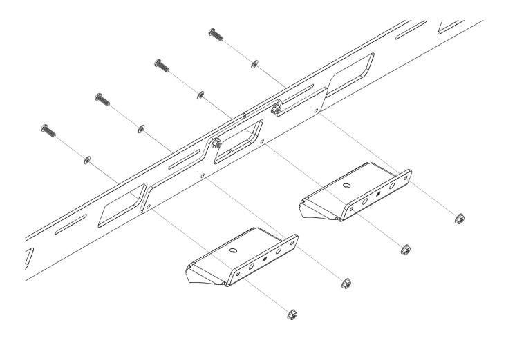
Next, attach the outer mounts. Start by loosely bolting them into the side rail using the 5/16"-18 X 1-1/2" hex head, .307/.327 ID washer, and 5/16" flange locknut. Make sure to get the gutter of the roof in between the inner and outer mounts.
