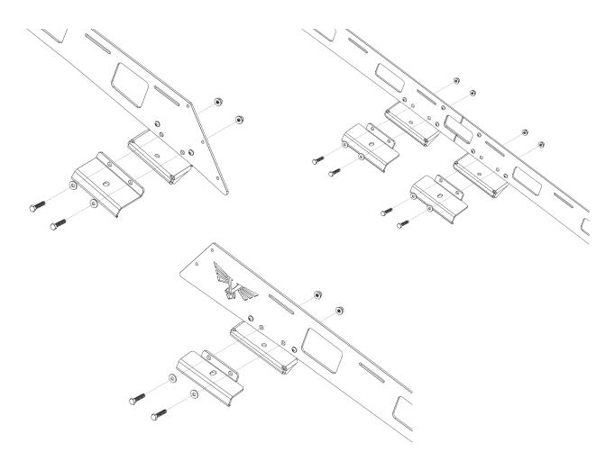
The outer clamps should be drawn into the inner mounts and secured to the drip rail using the (2)  $5/16'' \times 1 1/2''$  bolts and nylon locking nuts that pass thru the side rails. If the two mounts are too far separated initially to start the clamping hardware, a C-clamp or F-clamp can be used to pull the mounts together enough to get the hardware started.
