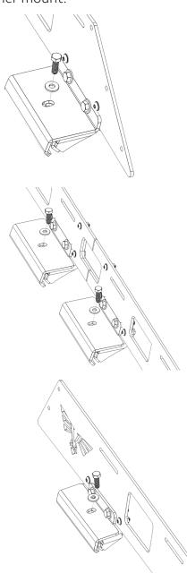
**10** Finally, push the front and rear fairings tight against the roof of the vehicle and tighten everything fully into place. We recommend applying clear 3M paint protection film to the roof of the vehicle anywhere the edge trim/ fairings make contact with the roof. This will protect the paint from dirt/ debris over time.
