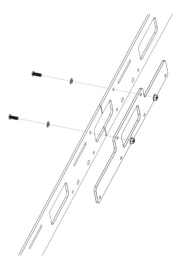
6 Next, lift the rack slightly and attach the mid mounts using the 1/4"-20 X 3.4" button head bolts, 1/4" ID washers, 1/4"-20 serrated flange nuts. Tighten them fully to the inside of the side rail.
