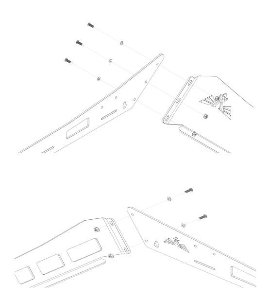
5 Next, attach the inner mounts to the inside of the side rails using the 1/4"-20 X 3/4" button head bolts, 1/4" ID washers, and 1/4"-20 serrated flange nuts. All of the mounts are identical, so it doesn't matter which goes where. Make sure that the side with the PEM nut on it is facing in, towards the center of the rack.
