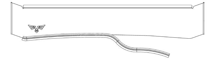
4 Next, mount the front and rear fairings. To do this, use the1/4"-20 X 3/4" button head bolts, 1/4" ID washers, and 1/4"-20 serrated flange nuts. The front fairing will need 3 of each per side and the rear fairing will need 2 of each per side. When mounting the front fairing, adjust it all the way up to avoid contact with the roof and leave the bolts loose enough to be able to make adjustments once it is on the roof of the vehicle.
