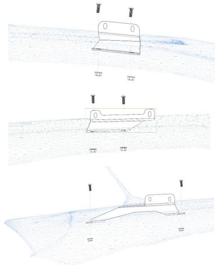
5 Next, put the assembled rack onto your roof and attach it to the mounts using the 1/4"-20 X 3/4" button head bolts, 1/4" washers and 1/4" serrated flange nuts. Make sure to keep the bottom edge of the rack an equal distance from the roof all the way down the length of the vehicle and tighten down fully.
