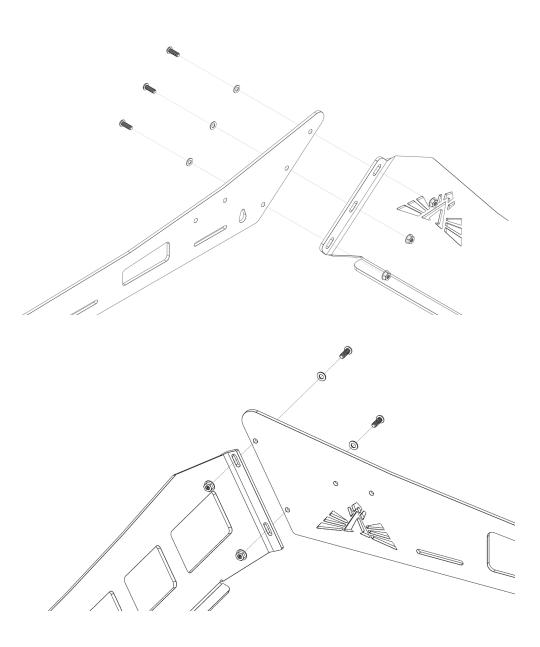
4 Next, attach the mounts to inside of the rack using the 1/4"-20 X 3/4" button head bolts, 1/4" ID washers, and 1/4"-20 serrated flange nuts.
