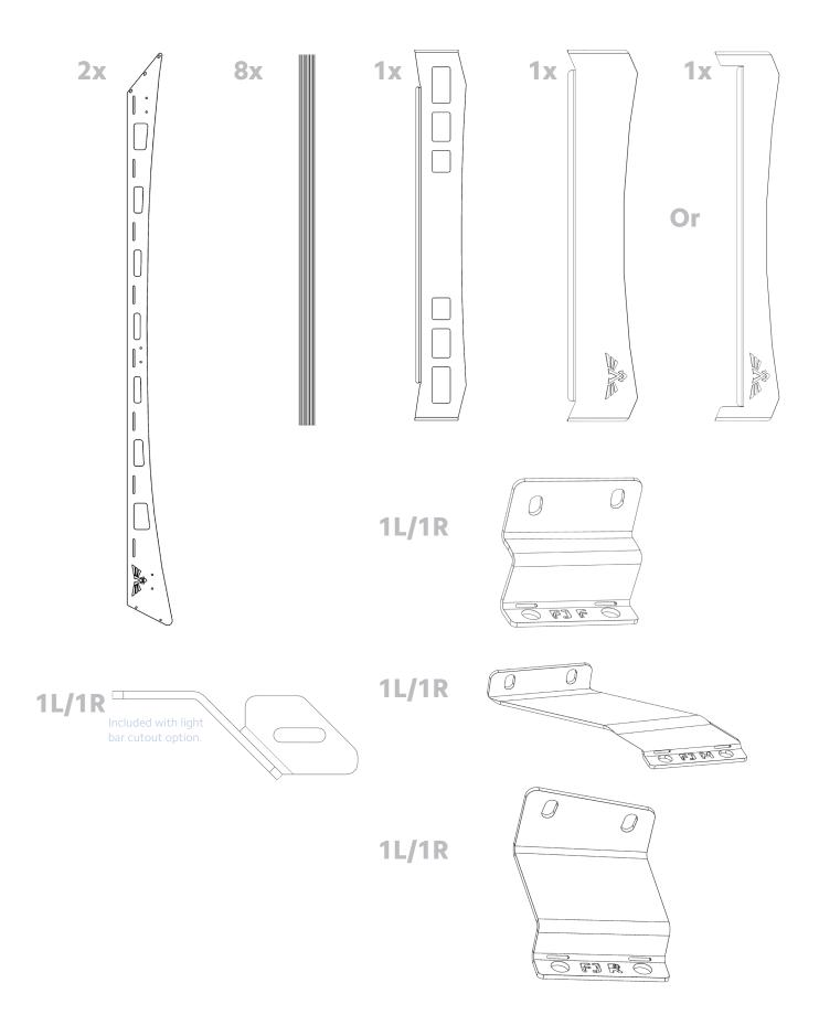
Assemble the rack on the ground. Start by mounting the crossbars between the two side rails. For this, use the 1/4"-20 X 3/4" button head bolts and the 1/4" ID washers (two per bar per side). Make sure the machined slot in the rail of the crossbar is facing up, so that you can easily add t-nuts to mount your gear.
