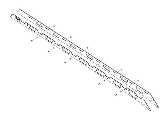
2 Assemble the rack on the ground. Start by mounting the crossbars between the two side rails. For this, use the 1/4"-20 X 3/4" button head bolts and the 1/4" ID washers (two per bar per side). Make sure the machined slot in the rail of the crossbar is facing up, so that you can easily add t-nuts to mount your gear.
