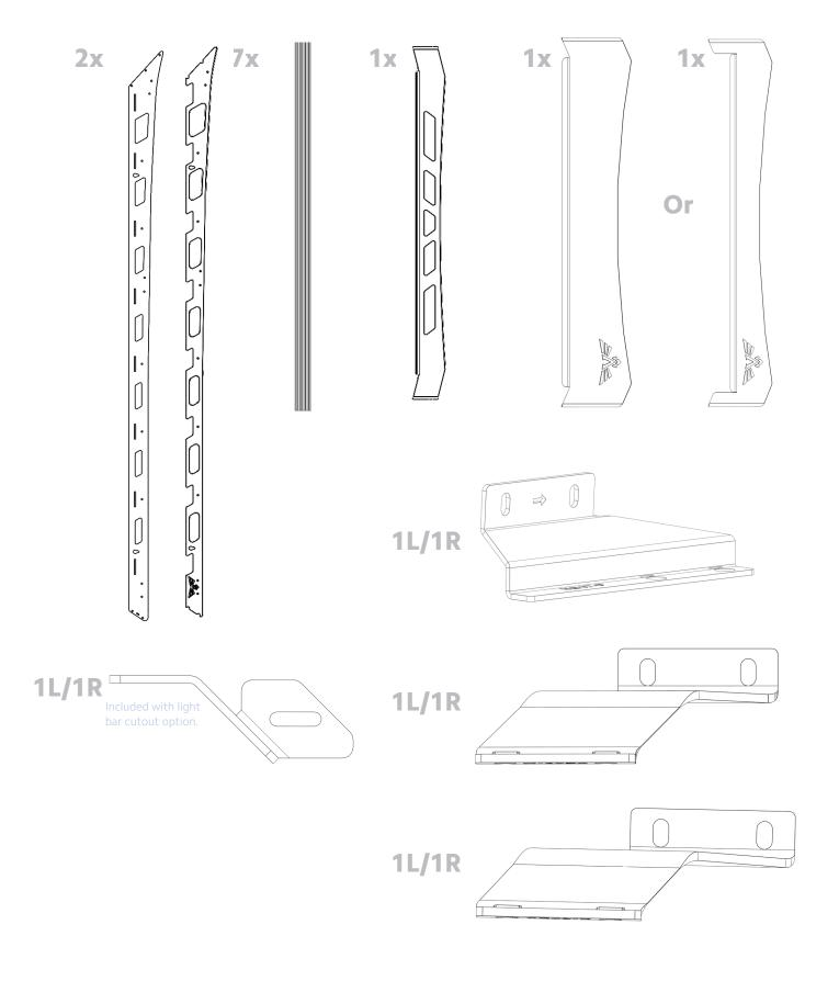
1 Assemble the rack on the ground. Start by mounting the accent plates to the side rails using the black 1/4"-20 nuts, black 1/4" washers and serrated flange nuts. The mounting holes are primarily the single holes located under the center of some cross bars. There will also be some unused mounting holes at the end of the installation that can be used to mount the accent plate. Use one bolt in the hole closest to the center of the crossbar above it.
