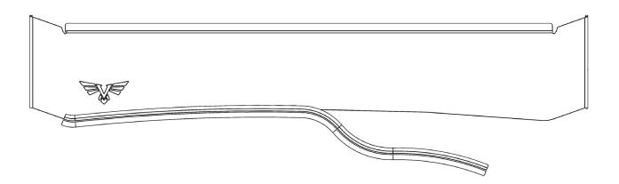
4 Next, mount the front and rear fairings. To do this, use the 1/4"-20 X 3/4" button head bolts, 1/4" ID washers, and 1/4"-20 serrated flange nuts. The front fairing will need three of each per side and the rear fairing will need two of each per side. When mounting the front fairing, adjust it all the way up to avoid contact with the roof and leave the bolts loose enough to be able to make adjustments once it is on the roof of the vehicle.
