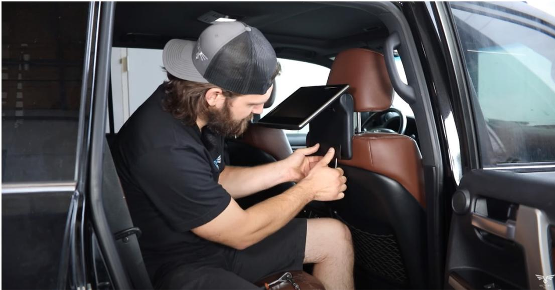
2. Once the plastic piece is popped off, you need to disconnect the (2) wire harnesses that are now exposed. Both should just be thumb tabs that you pinch to pop off. See below for the harness locations.
