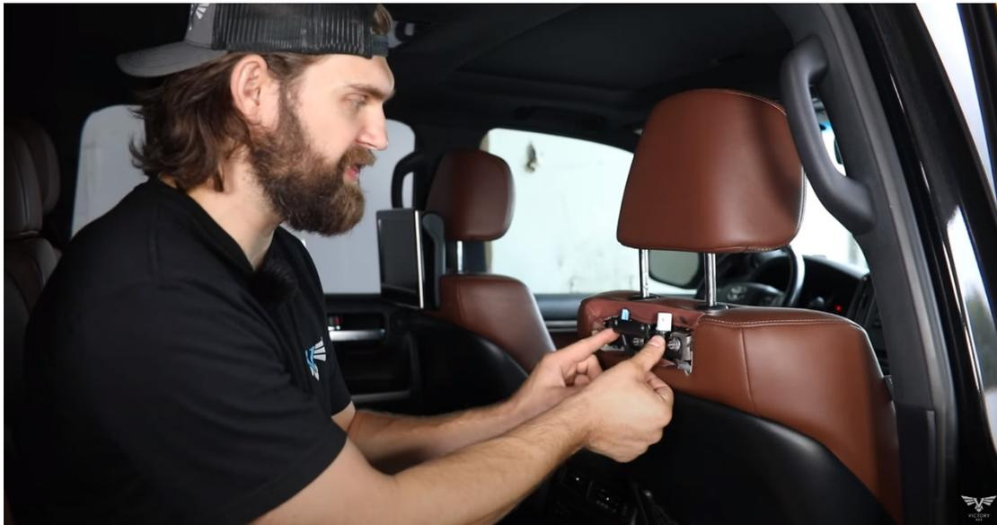
5. Once the bracket is secure and the wires are out of the way, take the provided button head bolts and use them to secure the face bracket to the mounting bracket, as shown in the orientation below, to complete your install. Repeat this same process for the opposite side.
