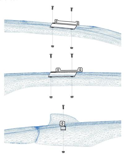
Next, put the assembled rack onto your roof and attach it to the mounts using the 1/4"-20 X 3/4" button head bolts, 1/4" washers and 1/4" serrated flange nuts. Once they are loosely attached to the rack, tighten the mounts fully to the roof. Then, make whatever adjustments to the rack that are necessary to get an even gap between the bottom edge of the side rails and the roof down the length of the vehicle and tighten the mounts fully to the side rails.
