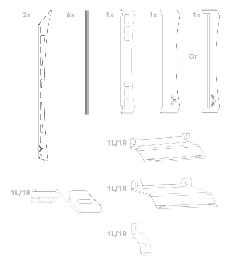
1 Assemble the rack on the ground. Start by mounting the crossbars between the two side rails. For this, use the 1/4"-20 X 3/4" button head bolts and the 1/4" ID washers (two per bar per side). Make sure the machined slot in the rail of the crossbar is facing up, so that you can easily add t-nuts to mount your gear.
