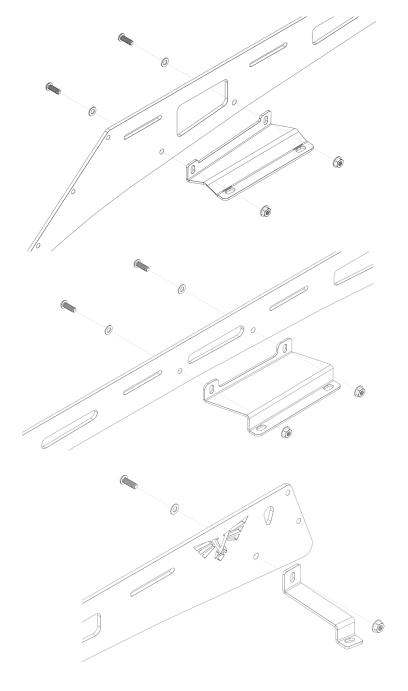
**6** Finally, push the front and rear fairings down tight to the roof of the vehicle and tighten everything fully into place. We recommend applying clear 3M paint protection film to the roof of the vehicle anywhere the edge trim/fairings make contact with the roof. This will protect the paint from dirt/debris over time.
