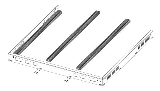
4 With all the bars loosely installed, bolt the final side panel on to all of them in the same way the third side panel went on. Before bolting it on, slide 6 T-nuts into the channel that is closer to the middle of the basket on each bar. These will be used to mount the floor panels.
