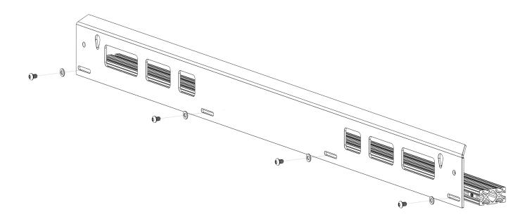
2 Next, attach a 3rd side panel to the ends of both cross bars. Line the slots on either end of it up with the 2 holes on each of the cross bars and bolt them together using the 1/4"-20 X 3/4" bolts and 1/4" washers. Leave the bolts loose for now.
