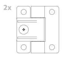
1 Start by loosely mounting the two hinges to the four slots in the bent bracket using the 1/4"-20 X 3/4" bolts, 1/4" ID washers and 1/4"-20 serr. flange nuts. It doesn't matter which side of the hinge as long as you put the flat side of the hinges on the bottom of the bracket. If you plan on using the friction adjustment on the hinge (the extra screw in the middle of one side) then it may be best to mount the side without the friction adjustment to the bracket.
