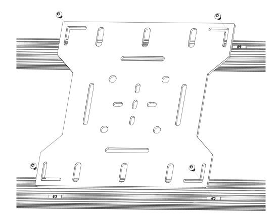
The accessory mount is made to be able to bolt on in many different positions. Depending on what gear you plan to mount on it, you may need to rotate the panel or even slide the crossbars forward or backward in their slots.
