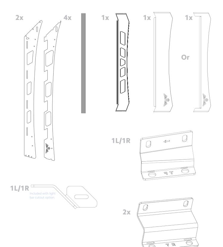
1 Assemble the rack on the ground. Start by mounting the accent plates to the side rails using the black 1/4"-20 nuts, black 1/4" washers and serrated flange nuts. The mounting holes are the single holes located under the center of some cross bars.
