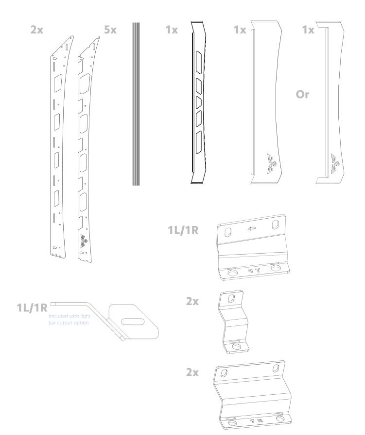
1 Assemble the rack on the ground. Start by mounting the accent plates to the side rails using the black 1/4"-20 nuts, black 1/4" washers and serrated flange nuts. The mounting holes are the single holes located under the center of some cross bars.
