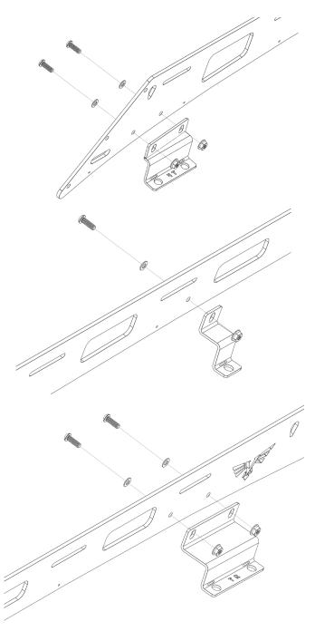
6 Next, apply RTV around the mounting holes on the roof of the vehicle and set the assembled rack into place. Try to get it as close to the correct position as possible so that you don't accidentally spread the RTV while trying to sliding the rack into position. Then, cover and fill the top of the mounting holes with more RTV so that the bolts will have to pass through it when tightening the mount in to place. Next, tighten it fully into place with the M6 bolts and M8 washers.
