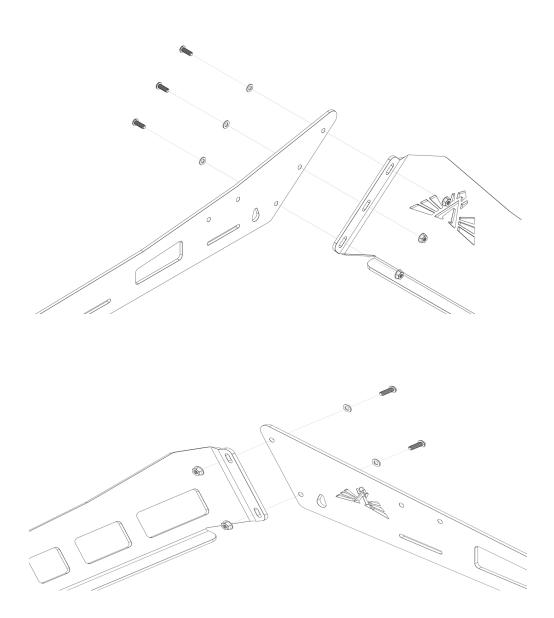
5 Next, attach the mounts to inside of the rack using the 1/4"-20 X 3/4" button head bolts, 1/4" ID washers, and 1/4"-20 serrated flange nuts. When attaching the front mount, make sure that the angled part of it is angled towards the front of the rack. The rear mounts are identical on both sides so they can be used on either.
