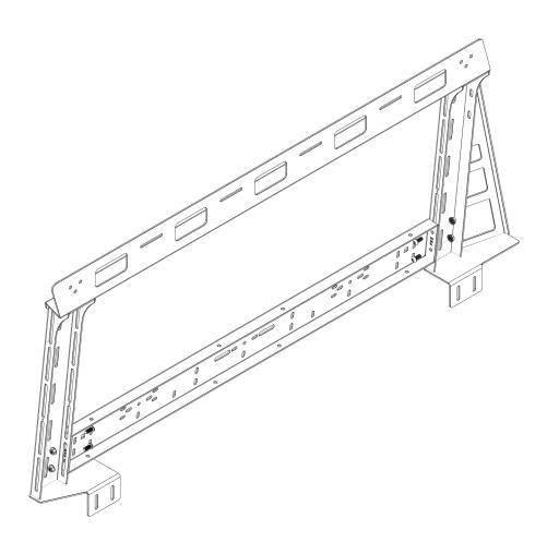
3 Next, connect the two sides you assembled together using the thinner cross bars with 5/16"-18 x 3/4" button head bolts and 5/16"-18 serr. flange nuts to mount them in position. One bar will mount to the front of the top rail, and one will mount to the rear. The open side should be on the bottom.
