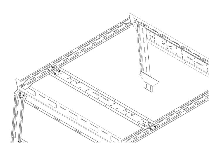
With the rack assembled, you can place it onto the bed of your vehicle. How you mount it depends on whether or not you have the trail rail system in the bed of your Gladiator. If you do, simply insert a 5/16"-18 x 1-1/2" carriage bolt through each hole in the small rectangular spacer and slide that into the trail rail. Do that three more times, then you can mount the legs of the bed rack using the 1/4" washers and 5/16"-18 flanged nylock nuts.
