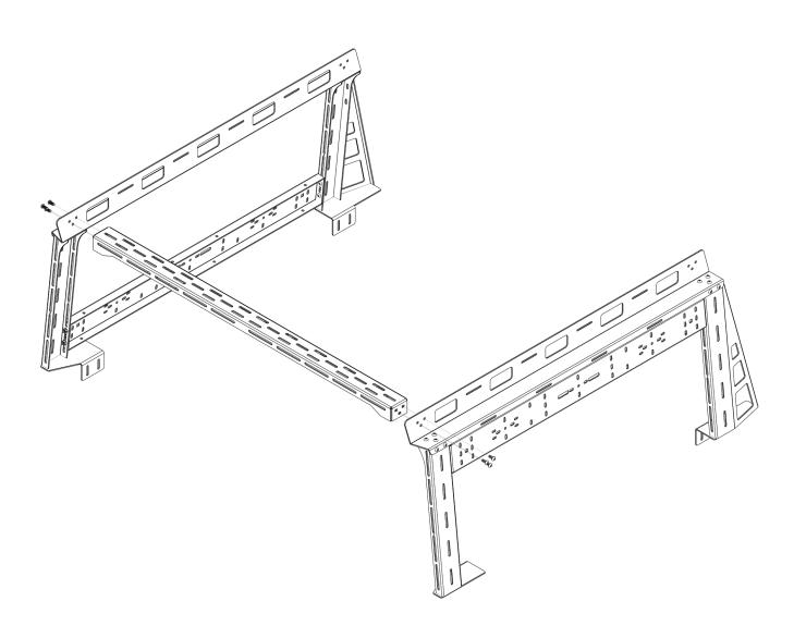
4 Next, mount the two remaining wider bars to the top of the rack between the bars you just installed. Do this using the 5/16"-18 x 3/4" button head bolts and 5/16"-18 serr. flange nuts. Which slots you mount them to is up to you and what you plan to use them for. Shown below is an image of the passenger side bar being installed from an underside view.
