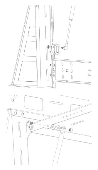
14 For the door opens down, attach one end of the lanyard to the hole in the middle of the leg using a 10-24 X 3/4" button head bolt, a #10 nylon washer and a 10-24 nylock nut. Then attach the other end to the inside of the door using the same hardware. Make sure the flat end of the eye of the lanyard sits against the nylon washer. The different holes in the door are there to give you options for how wide you want it to open.
