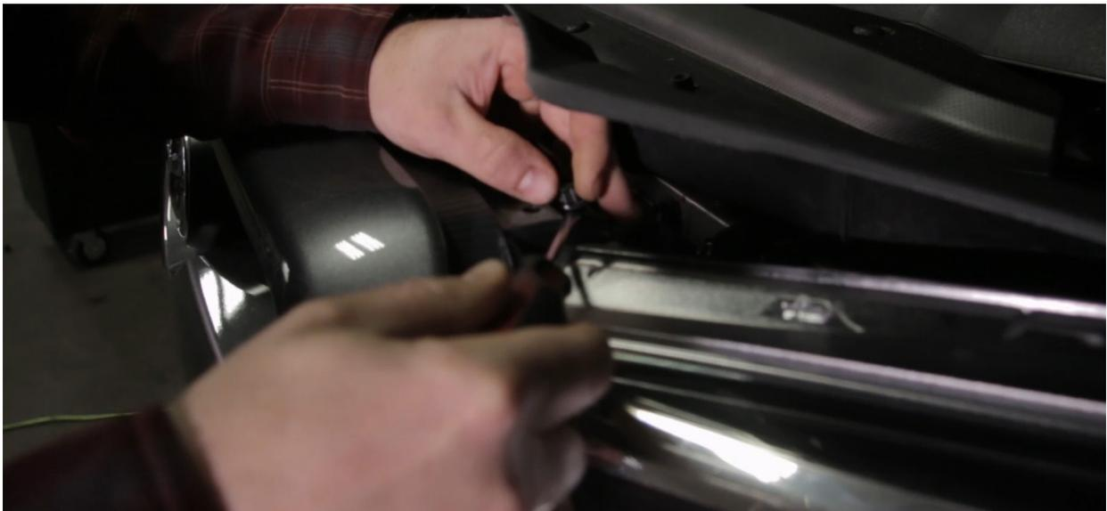
2. Use a 10mm socket to remove the bolt in the middle.
