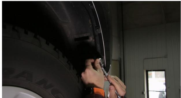
4. Remove the top part of the bumper by simply pulling the top portion off.
