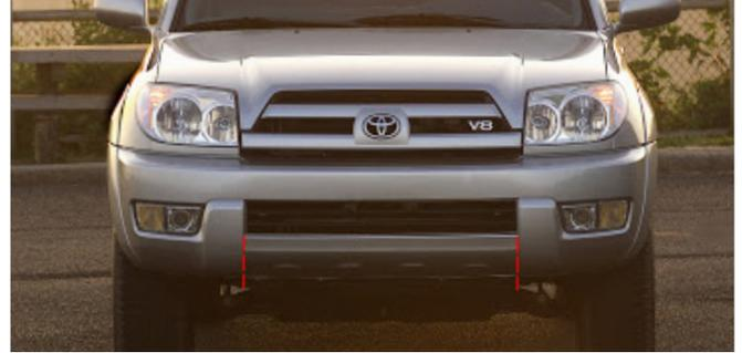
9. Use a 10mm socket and remove the 2 bolts on the bottom skid. Remove the bolts connecting the inner fender to the bumper bracket.
