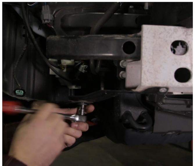
10. Use a 14mm socket and remove the bumper mounting bolts. There are 3 on the outside of the frame rail and 1 on the inside of the frame rail. Repeat the same steps on the other side. Remove the factory bumper and then reinstall the factory plastic cover we removed earlier.
