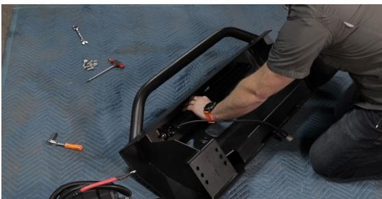
12. Install the winch. We will be installing a WARN VR 8-S. Loosely install the four mounting bolts under the bumper. Once they are loosely installed, flip the bumper over and tighten the mounting bolts. Next install the winch fairlead and tighten it down. Last we will tip the bumper forward and install the valance skid with the button head bolts we provide.
