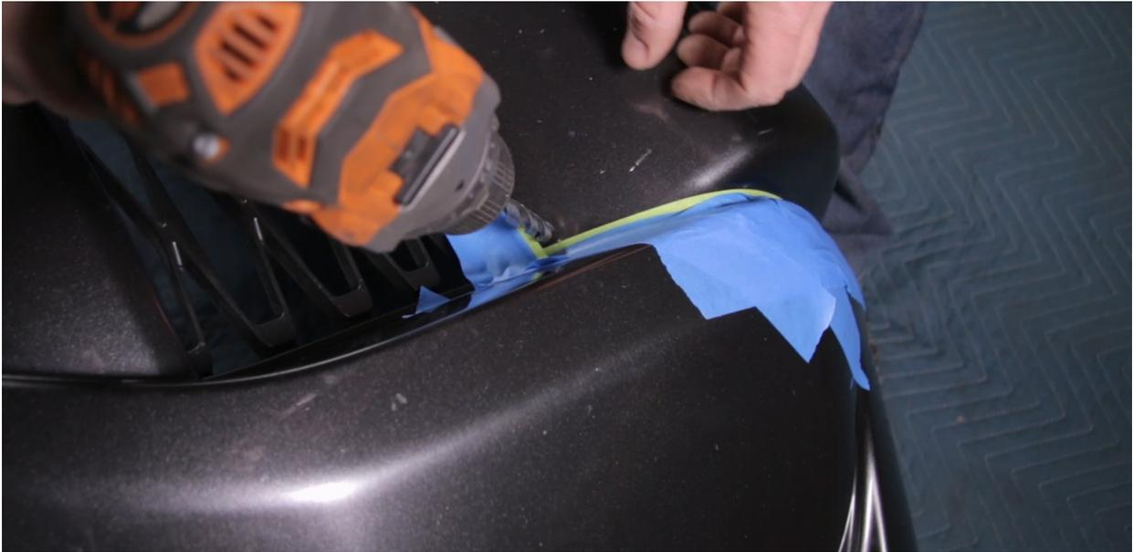
8. To cut the bumper we will be using a air saw with a round fiber cutting disk although there are many options for cutting tools. Use a sanding tool after you cut the line to smooth the edges. Remove the tape.
