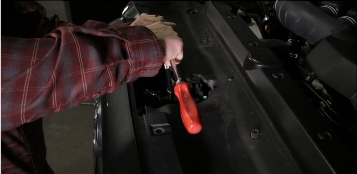
3. Remove all the bolts on the bottom that hold the bumper cover in place.
