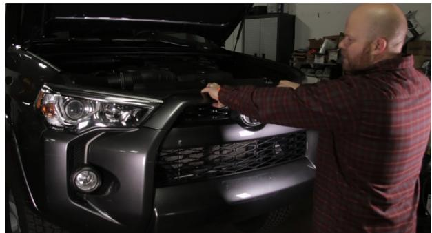
5. Remove the bumper. Gently pull the bumper away from the vehicle to release the snaps. Make sure not to pull the bumper completely off because the fog lights are still connected. Once you get 1 side loose, disconnect the fog lights so you can remove the entire bumper.
