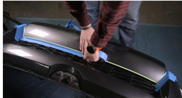
7. Drill a hole in the 2 corners of the front face bumper to create a smooth corner. We used a 3/8" drill bit.
