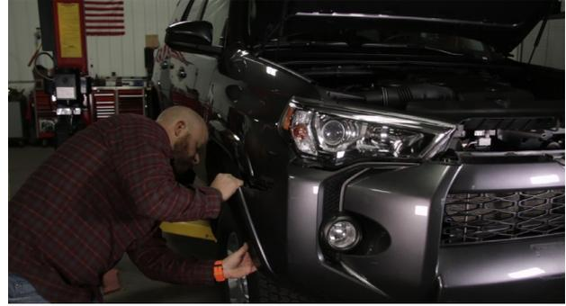
6. Place tape inside the curve of the bumper as shown in the picture below to make our cut line and to protect the paint. We will also be cutting the front face of the bumper so tape a line 3/8" down from the grill.
