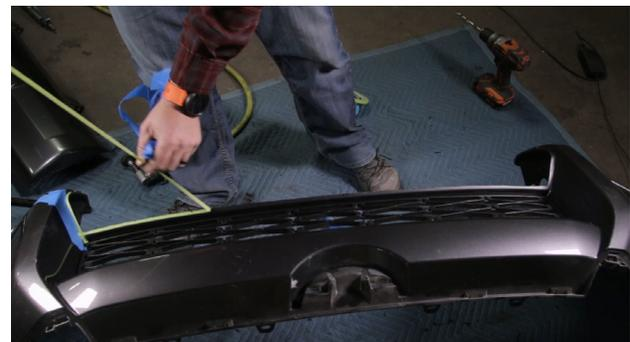
If you are installing a 4th gen (06-09) or (03-05) Blitz. You will cut along the red lines below and remove the lower portion of the factory bumper. The rest of the install will be the same.
