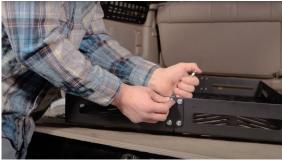
**4.** Install the supplied edge trim in each corner. Cut it into four 3" pieces. Use a non-marring plastic pry tool to open up the corner slightly and press the edge trim onto the side panel edge.
