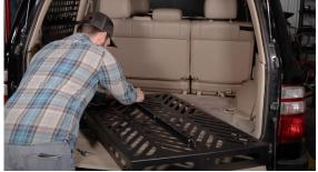
3. Flip the basket back over to install the tie-in brackets. Place the brackets on the outside of the basket and run the button head bolts through from the inside (this way the bolt ends don't protrude into the cargo area). Install all four bolts, washers, and flange nuts on each side loosely and then tighten them down.
