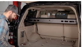
**6.** Bolt the basket to the brackets, dropping the bolts/washers through from the top with flange nuts on the underside. Start them all loosely first and then tighten them up with a 5/32" allen.
