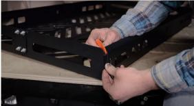
5. Carefully slide the basket onto the two side brackets, making sure you don't scratch the plastic interior trim near the hatch. On the 100 Series we are able to slide it straight in the back hatch. In other vehicles (i.e. 4Runner) you may need to fold the rear seats down and bring the basket in through the rear passenger door and slide it onto the brackets from the front.
