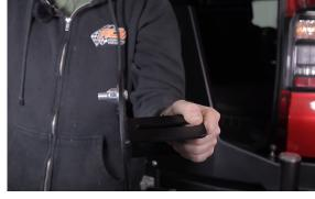
3. Loosely bolt the tire side of the mount to the carrier side using two carriage bolts and flange nuts.
