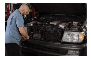
Remove the remaining bolts with a 10mm socket. There will be one on each side up through the bumper cover, into the fender. Then, remove the bolts on each tab along the underside of the bumper.
