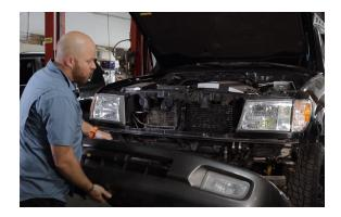
**3.** Remove the crash bar with a 14mm socket. With the bolts removed, you can lift the crash bar up and off of the frame.
