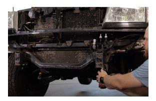
**5.** Install a clip nut in the hole on the top of the frame horns on each side using a hammer or mallet.
