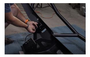
7. Set the bumper up on the frame and start a bolt down into one of the clip nuts you just installed to hold the bumper in place while you start the remaining bolts loosely. There will be three bolts on each side.
