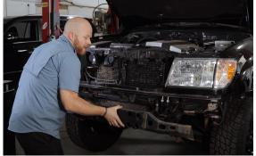
**4.** Remove the front tow hooks using a 21mm socket.
