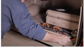
2. Using a panel tool or flat head screwdriver, pop the clips out as shown. There is one located below the door sill trim and one inside the jack storage compartment.
