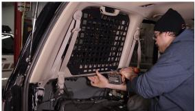
**9.** Next, the holes will need to be stepped up to 1/2" (through the plastic only) to fit the spacers. To do this, we will need to remove the panel.
