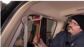
**6.** Bolt the upper bracket to the back of the MOLLE panel using button head bolts, washers, and flange nuts. Leave them loose for now.
