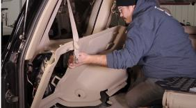
Unplug the wiring harness for the power outlet and then remove the panel and set it aside for now.
