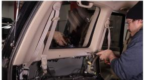
10. With those holes opened up to 1/2", double check that the spacers fit. You may need to open up the holes a little more. Ensure that the interior trim is fully snapped in and put the provided 1/2" spacers in the holes. The bolt pack will include to extra (larger) spacers that aren't needed. We will only be using the smaller spacers.
