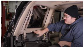
11. Reinstall the MOLLE panel. Push it tightly against the spacers aligning the holes in the spacers and the panel. Drill through the panel and spacer, through the metal. With one drilled, go ahead and bolt that one in place using a long button head bolt and flange nut. This will help hold the panel in place while you drill the second hole. With the second hole drilled, install a button head bolt and flange nut in that one as well.
