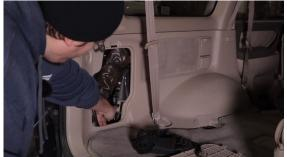
**3.** Continue to remove all the hardware holding the rear interior plastic in place. There is a T-20 screw to remove near the third row seat bracket. You can then remove that small panel.
