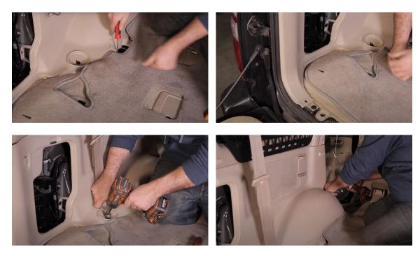
Put the storage cover back in place and reinstall the rear sill trim.
