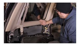
Pull the washer fluid line out of the clips and let it hang down out of the way.
