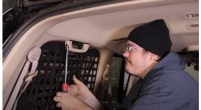
**8.** The next step will be to drill the lower two mounting holes. Press the bottom of the panel tightly against the interior trim. Using the panel as a guide, drill both holes with a pilot bit (through the plastic only at this point).
