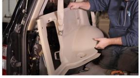
**4.** If you have the premium JBL sound system, you will need to remove the sub on the driver side. To do so, move the jack out of the way and remove the five bolts holding it in place using a 10mm socket.
