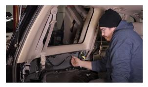
**5.** Remove the rear grab handle. Using a plastic pry tool, pop the covers off each side of the handle. Remove the Phillips screws under each one and set the handle aside.
