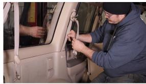
At this point, the whole panel will be held in with clips. Pull straight out and work your way around the edges to pop the panel off. Once it is loose tilt the top of the panel out to free the bottom edge from the carpet.
