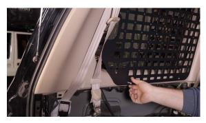
12. Tighten all of the hardware. If you have a sub to reinstall, you will need to leave the lower bolts loose in order to get it back up underneath. You may need to notch the upper tabs of the speaker housing to get it to fit without having to pop the trim back off.
