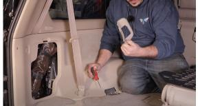
Next, remove the lower bolt for the third & second row seat belts using a 14mm socket.
