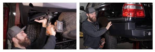
**10.** With the bumper fully installed, torque the rear M12 bolts to 70 ft/lbs and the lower frame M14 bolts to 110 ft/lbs. The rest of the hardware will just need to be tight.
