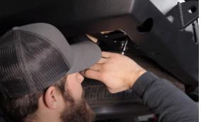
8. Now install the wing support brackets (shown off the vehicle below for reference). There will be three M14 bolts/washers into the frame, and two bolts/washers/nuts into the bumper wing. Get all of the bolts started loosely.
