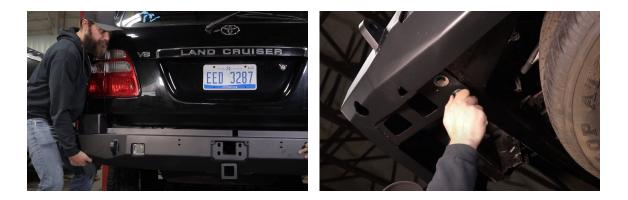
5. Start the two side frame bolts on each side by hand. (M8)
