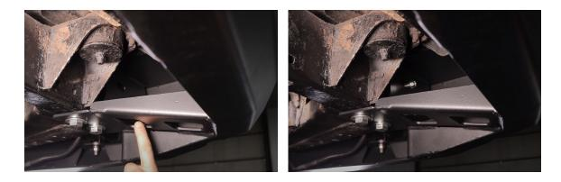
**6.** Start the four rear bolts loosely (M12). With all the bolts still loose, adjust the bumper left to right if necessary, checking clearance with the tailgate.
