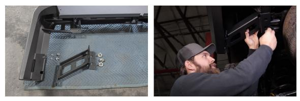
**9.** Tighten the frame-side bolts fully. With the wing-side bolts still loose, check that the body gap is even and make any minor adjustments to the wings that are necessary. Then tighten the wings.
