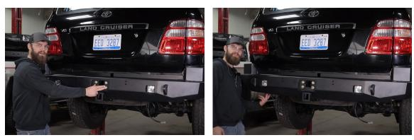
**11.** Install the cover plate using four button head bolts. Tighten with a 3/16" allen.
