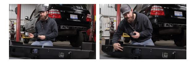
4. With the help of a friend, lift the bumper onto the vehicle. Start one a lower frame bolt (M14) & washer by hand to hold it in place. With it held in place, start the rest of the lower frame bolts/washers by hand.
