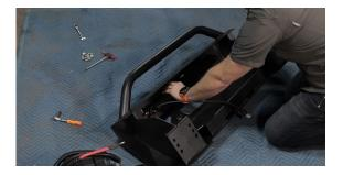
17. Mount the bumper. Have a friend help you or use a jack. Be sure to tuck the lower portion of the grill behind and under the top face of the bumper. Once you get the bumper mounted on the frame, loosely tighten the two inside bolts first, then tighten the three outside bolts on both sides. After you get all of the bolts loosely installed, tighten them down.
