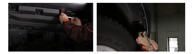
**4.** Remove the top part of the bumper by simply pulling the top portion off.
