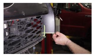
14. Next, trim the plastic bumper cover bracket near the fender. There is a metal bracket behind it that does not need to be cut, so be aware of that. You could mark the bumper line on the plastic bracket, remove it and then make the cut and reinstall it.
