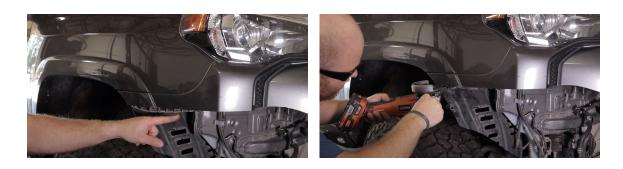
15. If installing a winch: loosen the bolts holding the cooling line in place and carefully bend the line toward the vehicle to make clearance for the winch. Use a 10mm socket and loosen the bolts holding the bracket in place. You do not need to remove the bolts.
