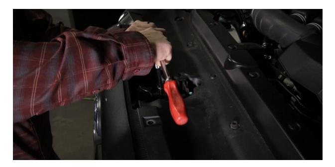
**3.** Remove all the bolts on the bottom that hold the bumper cover in place. You will also have to remove 3 bolts along the fender liner on both sides.
