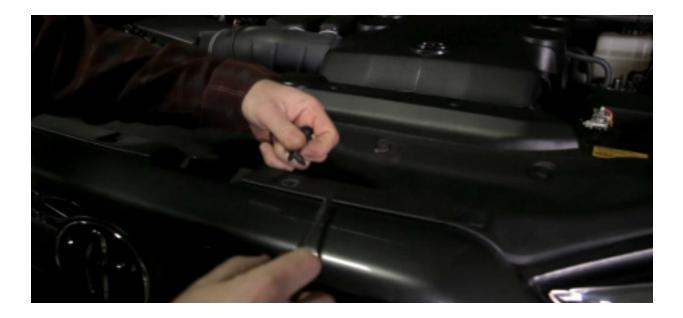
Once you remove the 4 clips, lift the cover up and remove 2 more clips. There is 1 clip on each side.
