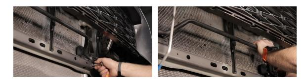
16. Assemble the Strike bumper. Start by installing a light bar or the aluminum filler panel and winch. If you are using a light bar you will need at least a 20" bar with a mounting width of 22". Cube lights can be installed now or after the bumper is installed
