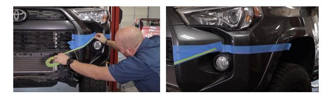
11. With the lines marked, it's time to make the cut. The cut will be only through plastic so you can use a sawzall, body saw, etc. We will be using a 4" cutoff wheel because it makes for a very straight line. Be careful, wear eye protection, and be sure to check behind the bumper for any wiring/ hard lines/etc. We found it was easiest to finish the cut through the fog light housing with a utility knife.
