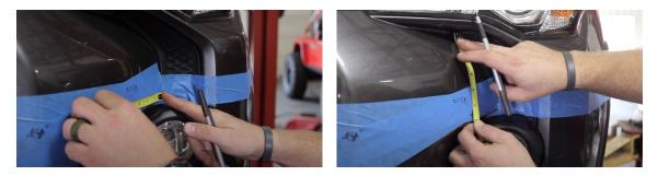
The third mark will be made by measuring straight down from the seam at the fender 1 1/2".
