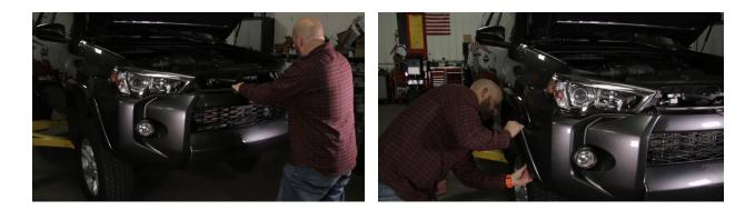
**6.** Use a 10mm socket and remove the 2 bolts on the bottom skid. Remove the bolts connecting the inner fender to the bumper bracket.
