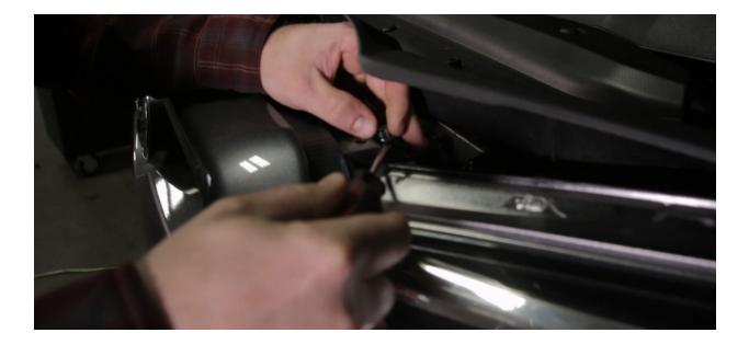
**2.** Use a 10mm socket to remove the bolt in the middle.
