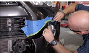
**12.** Clean up the cut with a flap wheel or sand paper and remove the tape.
