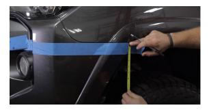
10. Now connect the marks with straight lines. This can be done one of two ways, by eye, using tape as a straight edge, or with a laser level (locked and adjusted). Repeat this process on the other side.
