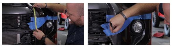
The second mark will be measuring horizontally from the edge of the fog light housing in toward the center of the vehicle 2 1/2" and down from the top corner of the fog light housing 5 1/2". Where those two lines meet will be our second mark.
