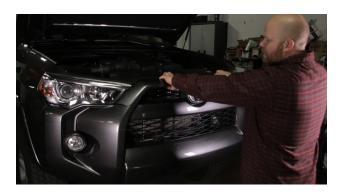
5. Remove the bumper. Gently pull the bumper away from the vehicle to release the snaps. Make sure not to pull the bumper completely off because the fog lights are still connected. Once you get 1 side loose, disconnect the fog lights so you can remove the entire bumper.
