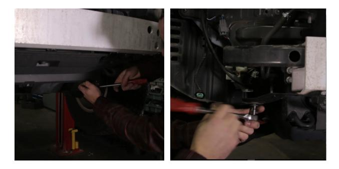
7. Use a 14mm socket and remove the bumper mounting bolts. There are three on the outside of the frame rail and one on the inside of the frame rail. Repeat the same steps on the other side. Remove the factory bumper and then reinstall the factory plastic cover we removed earlier.
