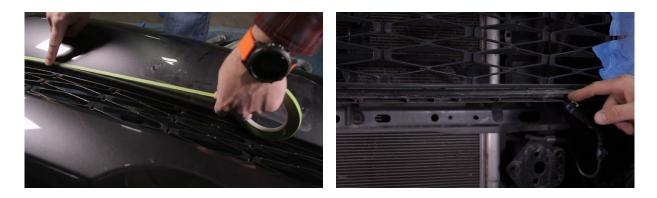
9. We will now make three measurements to mark the lines for the wing. The first will be 9 1/2" down from the bumper cover seam down to the corner of the bumper.
