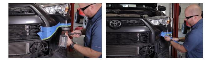
**13.** We will then make another cut with a utility knife on each side (as shown) to allow the bumper to slide in place. The top line will be straight back from the corner (parallel to the ground).
