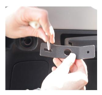
**3.** Remove the plastic cover over the front mounting location (inside the recessed area for the cargo cover) with a small flathead screwdriver or pry tool. Then remove the screw behind it.
