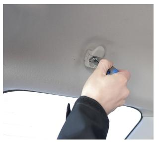
**6.** Put the hanger through the bracket and reinstall using the stock hardware.
