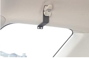
7. With all three mounting brackets loosely installed, hang the panel using two 1/4" button head bolts and flange nuts.
