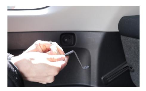
**5.** Pop the cover off of the hanger hook with a pry tool and remove the screw.
