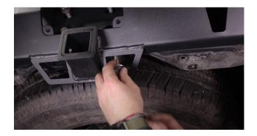
**18.** Once all of the bolts have been started by hand and the bumper is aligned, go ahead and tighten them down. The M8 bolts will use a 12mm socket and the M12 bolts will use a 19mm socket.
