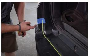
3. The next step will be to mark the line on top of the rear bumper. Follow the seam on the bumper all the way to the corners. You can measure 1/4" from this line or use 1/4" tape and follow the line in the bumper exactly. We will then make our cut on the outside edge of the tape. When the line on the bumper ends, continue your tape straight up to your first line (blue tape).
