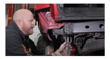
**9.** Next, install reverse lights (3"x3"), if you plan to run them, now. They can not be installed once the bumper is installed.
