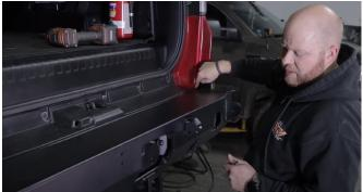
16. Now install the rest of the frame mount bolts loosely. Start with the two rear M12 bolts and washers. Then start the three front M8 flange head bolts. You may have to move the bumper around slightly to get all of the holes aligned. Once they have all been started finger tight, do the same on the other side.
