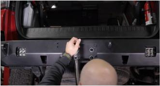
20. Reinstall the rubber exhaust hanger.
