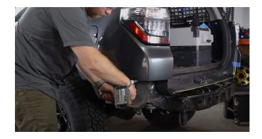
**7.** Remove the hitch receiver with a 17mm socket or wrench. There are four bolts on the back and two underneath.
