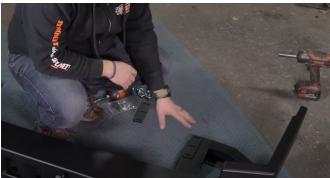
13. Remove the rubber exhaust hanger. Spray the mounting holes with a lubricant and then pry it off using two pry bars or large screwdrivers. Then fold the rubber hanger down and let it hang for now. We will reinstall it later.
