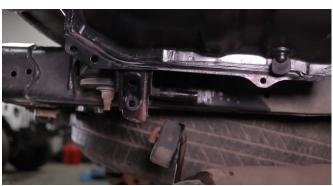
14. With the help of a friend, lift the bumper up into place. On the passenger side, you will need to slide the bumper mount between the exhaust and the frame. With the bumper in place and both of you still holding the bumper, loosely install the four M12 bolts above the hitch. Now the bumper will be supported and you can work on the bottom mounts.
