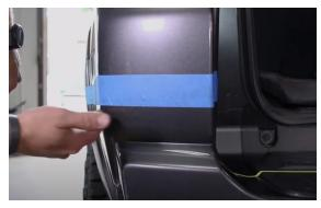
To ensure the line is straight around the corner of the bumper, measure up 2.25" from the body line as shown below. If you have a Limited or 10-13 model, you won't have this hard body line. You can check your line by measuring down from the bottom of the tail light 8.75". Continue this line, inside behind the hatch, straight back as shown.
