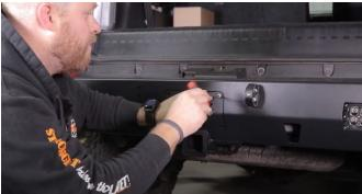
22. If you are not installing an Adventure Carrier now, install the plastic caps on the top and bottom of the spindle sleeves. Use some black RTV to keep them in place and keep water out. This will keep the spindle sleeves clean and allow you to install a carrier or carriers later on!
