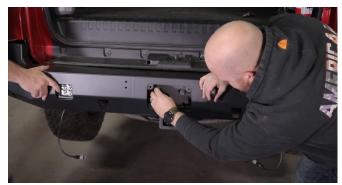
15. Make sure that the lip of the remaining stock plastic bumper (under the hatch) is underneath the Strike Bumper. If not, you should be able to wiggle the bumper and press it underneath now. Also check to make sure the bumper is centered and the notches in the Strike bumper are around the vertical cuts on the factory plastic.
