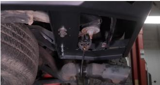
**21.** Install the cover plate using four 5/16" button head bolts and washers. We recommend putting some anti-seize on the threads. Tighten them down with a 3/16" allen.
