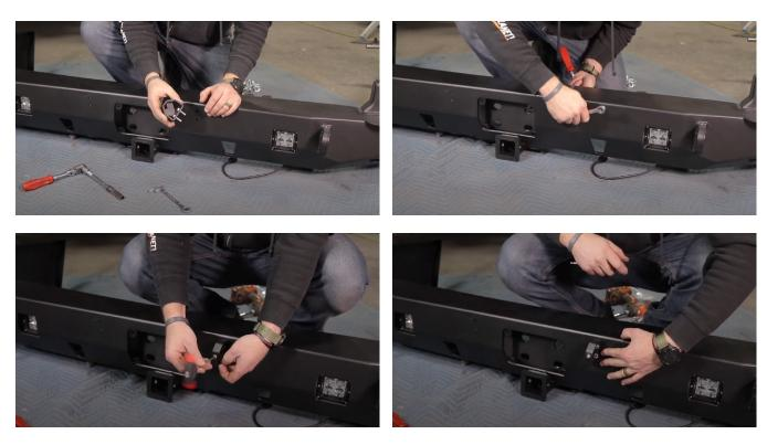
Be sure that these bolts do not come loose over time as they are what will hold the carrier(s) closed. You can use Red Loctite here.
