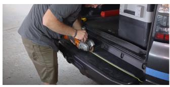
**5.** Once the cut is done, there are two bolts to remove under the plastic bumper, near the hitch. The bumper and foam can now be removed.
