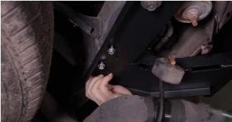
17. Start the two M12 bolts underneath the bumper up under the chain hangers on either side of the hitch receiver.
