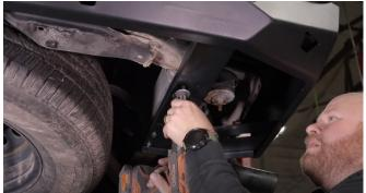
**19.** Now torque the bolts. Torque the M8 bolts to 20-25ft-lbs and the M12 bolts to 60ft-lbs.
