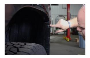
The next step will be to mark the cut line on the factory rear bumper. Measure down from the body line 5", as shown, in two places, one by the wheel well and the other just before the line turns up to the tail light. Connect these two marks with a straight line and continue it around the corner where we will make another mark. You can connect the marks using tape as a straight edge or you can use a laser level (locked) as a straight edge.
