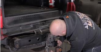
**8.** Remove the factory tow hook with the same 17mm socket or wrench.
