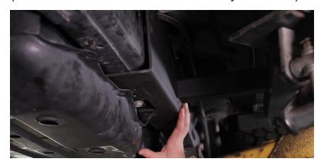
7. With your slider in place, begin loosely installing bolts into the mounting holes. Once you get all of the bolts installed, tighten the bottom bolts (Image 2) to bring the slider against the frame before tightening the other bolts. Once the bottom bolts are tight, go back and tighten the rest of the bolts. If you have KDSS, you will bolt it back on over the slider mounting plate.
