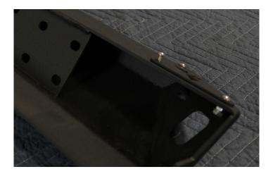
2. Now bolt the legs onto the slider. The outer portion of the sliders are symmetrical. The only difference between sides will be how the legs are positioned. Both legs will be bolted in the front-most set of holes. (closest to the front of the vehicle). There will also be an arrow cut in the mounting plate of each leg pointing toward the front of the vehicle. Once you have them positioned, install them using the provide button-head bolts and flange nuts. Do not fully tighten them yet.
