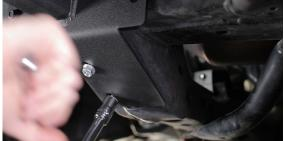
**11.** You will find one bolt hole on the passenger side that is smaller than the others. Once you find the smaller hole use a self-tapping bolt to secure it.
