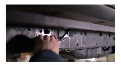
**5.** Remove the three bolts holding the gas tank skid in place. Then remove the bolt holding up the brake line and any other lines (KDSS if you have it).
