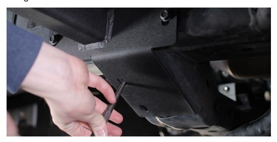
10. Once the two holes are drilled, use two 3/8" self-tapping bolts with a 9/16" wrench to secure the bolts. (do not over tighten them, just until they are snug)
