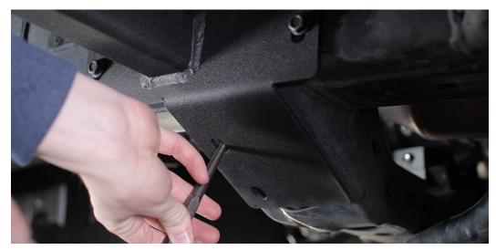
**6.** Once the two holes are drilled, use two 3/8" self-tapping bolts with a 9/16" wrench to secure the bolts. (do not over tighten them, just until they are snug)
