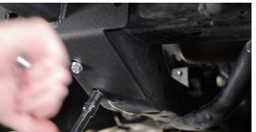
7. You will find one bolt hole on the passenger side that is smaller than the others. Once you find the smaller hole use a self-tapping bolt to secure it.
