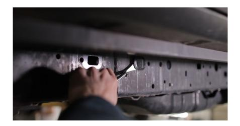
2. Remove the three bolts holding the gas tank skid in place. Then remove the bolt holding up the brake line and any other lines (KDSS if you have it).
