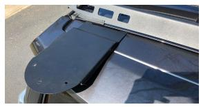
**3.** Now set the ladder on top of the bracket you just installed, place a towel between the bottom of the ladder and tailgate for now to protect the paint. Start the three bolts and flange nuts and snug them up.
