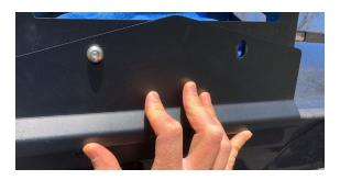
**6.** Press the bottom bracket firmly against the bottom of the hatch so it sits flush. Drill the two bottom holes through the bracket using a 5/16" drill bit. Once the holes are drilled, you can remove the bracket and touch up the holes with paint to prevent rusting.
