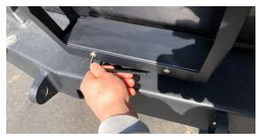
**9.** The top and bottom brackets are slotted front to back, so go ahead and adjust the depth/angle of the ladder if you need to and tighten down all of the bolts. Enjoy your new ladder!
