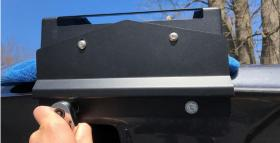
**8.** Install the bottom step using two button head bolts and flange nuts. Make sure that the back flange of the step is sitting on top of and over the back of the ladder. Once installed, fully tighten the step.
