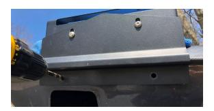
7. Reinstall the bracket and use the two hex head bolts, washers, and flange nuts to install the bottom to the hatch. You can reach through the handle hole to start the nuts. They are serrated flange nuts, so once they are started, you shouldn't need a wrench on the inside. You can now fully tighten these two bolts using a 1/2" socket.
