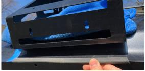
**5.** Now loosely install the bottom bracket with two button head bolts and flange nuts.
