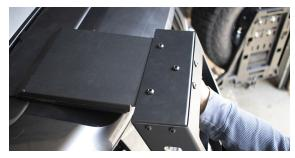
8. Place a level on the side of the ladder to ensure correct positioning to drill the bottom mounting holes. Once you have the ladder aligned where you want it, mark the position of the bottom of the ladder with tape. Place the two small pieces of edge trim on the hatch, directly below the ladder.
