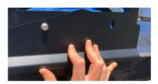
Press the bottom bracket firmly against the bottom of the hatch so it sits flush. Drill the two bottom holes through the bracket using a 5/16" drill bit. Once the holes are drilled, you can remove the bracket and touch up the holes with paint to prevent rusting.
