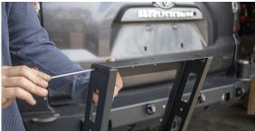
**6.** Bolt the steps into the ladder using button head bolts and flange nuts. The two lower steps will be identical, the top step rear-flange will be angled (see photo below for reference). The flange side will go toward the back of the ladder.
