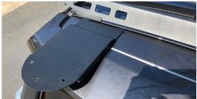
**3.** Now take the ladder and flip it upside down. Take the step and install it with two button head bolts and flange nuts, sliding it in through the bottom of the ladder. Leave the bolts loose.
