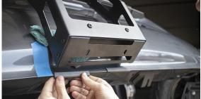
**9.** Now loosely install the bottom bracket with two button head bolts and flange nuts.
