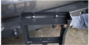
**4.** Install the bottom plate over the step as shown. Bolt it in with four button head bolts and flange nuts. Tighten all six bolts now.
