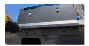
Reinstall the bracket and use the two hex head bolts, washers, and flange nuts to install the bottom to the hatch. You can reach through the handle hole to start the nuts. They are serrated flange nuts, so once they are started, you shouldn't need a wrench on the inside. You can now fully tighten these two bolts using a 1/2" socket.
