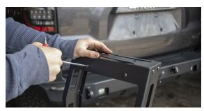
**5.** Now flip the ladder right side up and install the top plate with six button head bolts and flange nuts. Tighten them fully.
