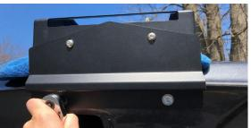
12. The top and bottom brackets are slotted front to back, so go ahead and adjust the depth/angle of the ladder if you need to and tighten down all of the bolts. Enjoy your new ladder!
