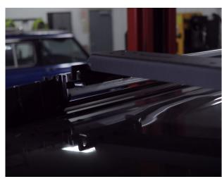
**4.** Loosely install all of the lock nuts and adjust where you want the crossbars to be placed from front to back.
