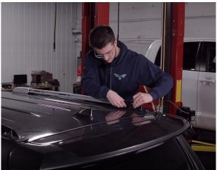
**3.** Once the brackets are roughly in place, install the crossbars. Put the carraige bolts through the side of the crossbar with holes and then the opposite side with slots can drop onto the carraige bolts on the other side.
