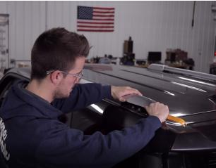
2. Put two carriage bolts in each mounting bracket. You will need one per side, per crossbar. Slide the brackets in the side rails on each side.
