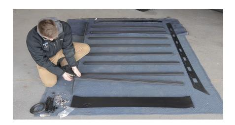
2. Mount the front and rear fairing. Use the small button head bolts along with the small washers and a flange nut. Adjust the fairings all the way up, for now, to avoid contact with the roof when you set the rack in place.
