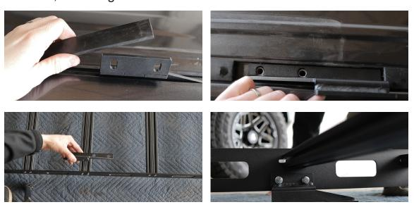
**6.** Install the rear mounts with the V-shape facing upward. Use 2 button head bolts, washers, and flange nuts.
