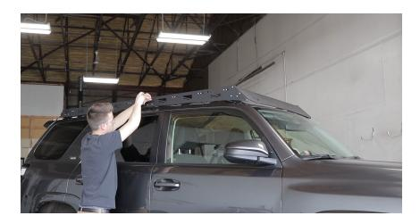
**10.** Use the trim we provide and cover the lower part of the front fairing (approx. 41 inches). Use the remaining trim on the back. We recommend cutting it in half and placing the trim on either end of the back fairing.
