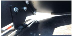
5. Lift the factory rubber so you can place the middle mount and see where you'll have to trim it. Then install the middle mounts onto the rack with the long end facing toward the front of the rack. Use 2 button head bolts, washers, and flange nuts.
