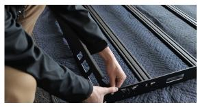
3. Use a pry tool to remove the 4 caps on the stock rails. Use a 12mm socket to remove the bolts holding the rails in place.
