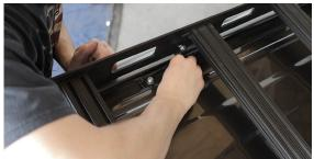
**9.** Once you have the hardware tight on the roof you can tighten the hardware on the side rails and the crossbars using a 5/32 allen.
