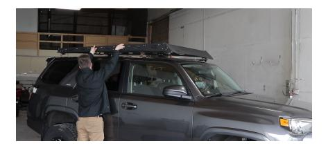
**8.** With the rack in place, use RTV and spread it under the mounts and fill the bolt holes. Use the larger bolts and washers to secure the rack to the roof using a 3/16 allen. You should see RTV squeeze out under the bolt heads when you tighten them, this will prevent any leaking. Be sure not to over tighten the mounting bolts.
