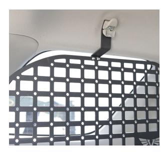
8. Now attach the remaining two holes with 1/4" button head bolts and flange nuts. Once it is all loosely bolted together, level the panel and tighten all of the bolts down. Don't forget to clip the cover back on the hanger and pop the cargo net hook into the new bracket.
