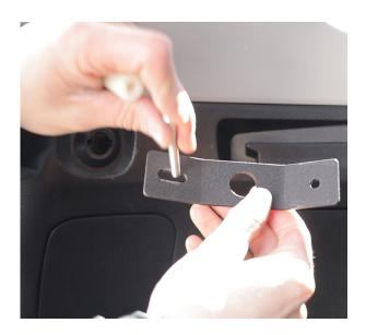
**3.** Remove the plastic cover over the front mounting location (inside the recessed area for the cargo cover) with a small flathead screwdriver or pry tool. Then remove the screw behind it.
