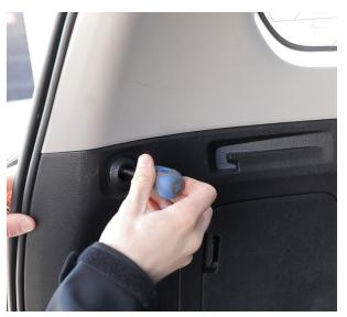
2. Now loosely install the rear bracket with an M6 Button Head and spacer, like so.
