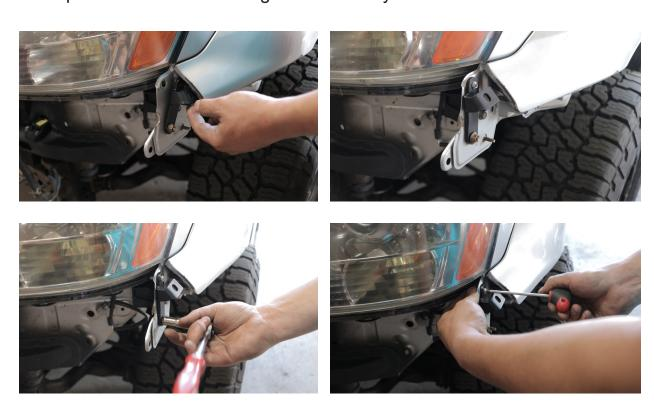
11. Install the filler panels on the brackets using the hardware provided.
