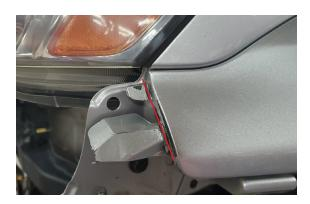
**9.** Remove the plastic bracket below the fender using a 10mm socket and trim the plastic on either side as shown. This will make room for the bumper wings.
