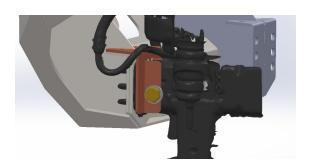
**16.** Install the bumper on the frame studs using the factory hardware. Tighten down with a 14mm socket.
