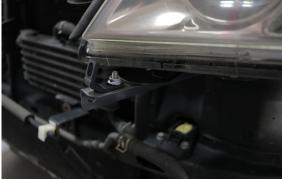
8. Trim the plastic tabs off below the headlight at the fender as shown.
