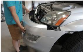
**4.** Remove the bumper support bracket with a 10mm socket.
