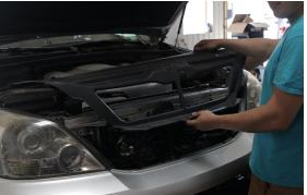
2. The next step will be to remove the factory plastic bumper. Start by removing the retaining clips along the top with a trim tool.
