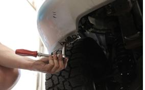
**3.** Pull the bumper outward at each wheel well to unclip it, then pull the bumper straight off from the front.
