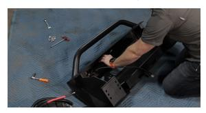
13. Install the winch. We will be installing a WARN VR 8-S. Loosely install the four mounting bolts under the bumper. Once they are loosely installed, flip the bumper over and tighten the mounting bolts. Next install the winch fairlead and tighten it down. Last we will tip the bumper forward and install the valance skid with the button head bolts we provide.
