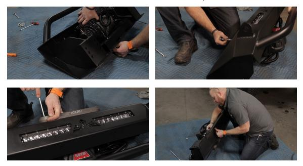
14. Loosen the bolts holding the cooling line in place and carefully bend the line toward the vehicle to make clearance for the winch. Use a 10mm socket and loosen the bolts holding the bracket in place. You do not need to remove the bolts.
