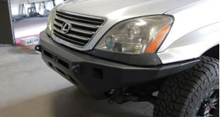
17. Put a bolt through the top of the tie-in bracket & bumper to locate the bracket on the frame. Drill a 5/8" hole through the side of the bracket & frame rail. Touch up any exposed metal with paint and install all of the supplied hardware.
