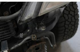
7. Install the inner filler plate brackets in the holes you just drilled, using the hardware provided.
