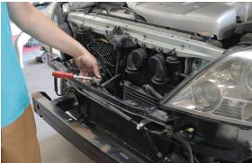
**5.** Remove the crash bar with a 14mm socket.
