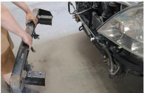
6. The next step will be to measure and drill an additional hole in the remaining bumper support bracket on each side (under the headlights).
