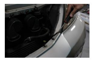
Remove the remaining bolts with a 10mm socket. There is one in each wheel well and seven underneath the front of the bumper.
