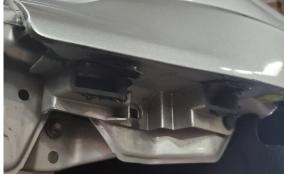
10. Install the outer filler plate brackets (one on each side). The lower hole will mount using a factory stud and nut, use the supplied hardware to mount the top hole. Go ahead and tighten them fully.
