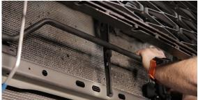
**15.** Place the tie-in brackets over the frame horns. We will mark/drill them after the bumper is installed.
