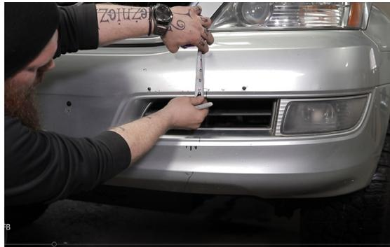
2. Now mark the side of the cut. There will be three measurements to make. The first will be just inside the fin again, this time underneath. To mark this accurately, you can measure 9" from the center-most body line (as shown). The second measurement will be 10" straight across from that same body line. The bottom measurement will be 9", again from that same body line. Connect all of your marks with sharpie or tape.
