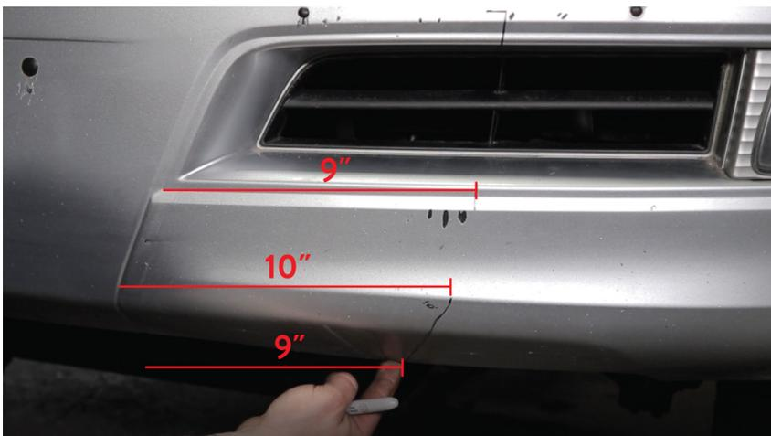
3. Repeat this process on the other side and connect your top marks with a straight line. We are using a laser level, locked, so we can use it as a straight edge. You won't want the level free floating because your truck might not be level.
