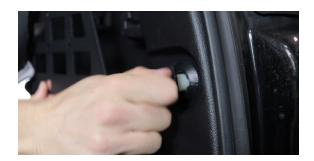
**10.** Tighten the C bracket behind the panel using a 5/32 allen. Once the bracket is tight, you can secure the panel to the bracket using a button head bolt and flange nut.
