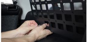
**11.** Tighten the C bracket behind the panel using a 5/32 allen. Once the bracket is tight, you can secure the panel to the bracket using a button head bolt and flange nut.
