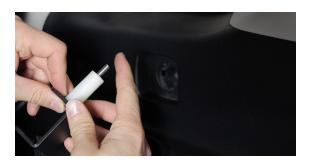
**6.** Remove the right side bolt from the handle. Squeeze the side of the handle and pull back on the plastic cover to expose the 10mm bolt.
