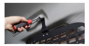
9. Next we will install the rear bracket. Use a spacer and the long button head bolt. Make sure the seat belt is in front of the panel and not behind it.
