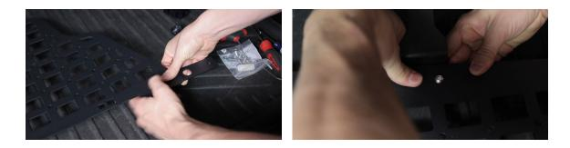
**8.** Now we can install the panel. Start by hanging the panel from the top bracket. Use the 10mm bolt we removed earlier and secure it to the handle.
