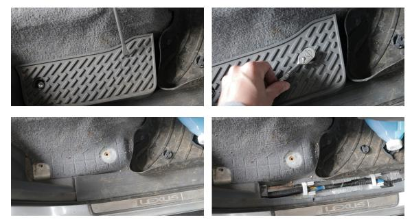
**4.** Remove anything else attached to the rear interior panel, power outlet, seatbelt bolts, etc.
