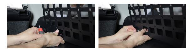
**11.** Tighten the C bracket behind the panel using a 5/32 allen. Once the bracket is tight, you can secure the panel to the bracket using a button head bolt and flange nut.
