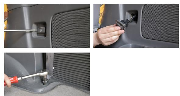
5. Now pop the interior panel out. You will need to pry the plastic up past the third row seat mechanism with a screw driver or pry tool so it can slide up and over.
