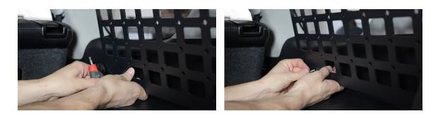
**12.** Reinstall the seat belt clip and cargo net hook to the panel. Go back and tighten everything down and you will be finished with the install.
