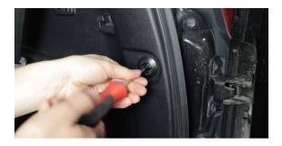
**3.** Remove the seat belt clip. Press in the tabs holding it in with a flat head screwdriver
