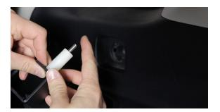
**6.** Remove the right side bolt from the handle. Squeeze the side of the handle and pull back on the plastic cover to expose the 10mm bolt.
