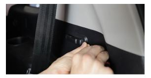
**4.** Remove the small panel below the window. Then remove the phillips head screw that the panel was covering up.
