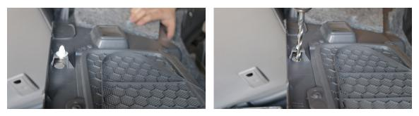
**7.** Open up the two holes that the white clips clipped into with the included 24/64" drill bit. Install two nutserts into the metal.
