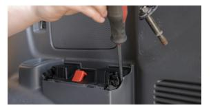
**6.** Remove the two white plastic clips from the back of the panel. Use those clip locations to drill through the panel with a pilot bit. This will mark the hole locations on the front for the nutserts.
