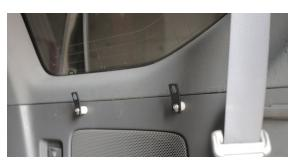
**11.** Remove the grab handle by prying off the caps and removing the bolts using a 10mm socket.
