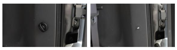
**2.** Remove the hatch sill trim using a phillips head screwdriver. Once the screws are removed, it will just be held in with clips and can be popped out.
