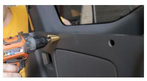
**10.** Install the spacers, bolts, and lower brackets through the plastic and into the nutserts as shown.
