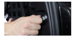
**10.** Tighten the C bracket behind the panel using a 5/32 allen. Once the bracket is tight, you can secure the panel to the bracket using a button head bolt and flange nut.
