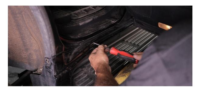
**3.** Pry up the plastic step plate with a flat head screwdriver or pry tool and remove it.
