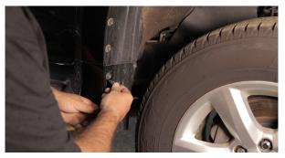
**8.** Next, mark the trim to be cut. In the front, measure from the top of the trim down 3.25" and tape straight across from front to back. In the rear measure down 2" and mark with tape.
