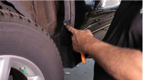
2. Remove the two phillips head screws in the door sills. You will need to open the doors to do this.
