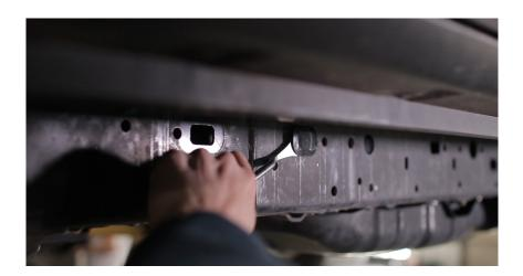
**14.** Remove the three bolts holding the gas tank skid in place. Then remove the bolt holding up the brake line and any other lines (KDSS if you have it).
