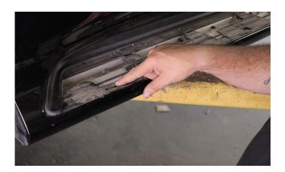
**5.** Unplug the wiring harness and unbolt the steps from the body. There are two 12mm bolts on each of the three mounting brackets.
