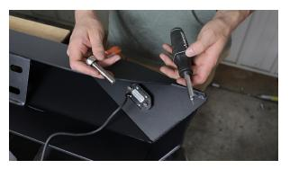
11. Bolt the legs to the slider using the large button heads and flange nuts. The front mounts are the smaller of the two. Each leg will have an arrow cut into the mounting plate, pointing toward the front of the vehicle.
