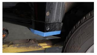
**10.** Assemble your new Blitz Sliders. Start by installing the LED lights using the provided button head bolts, washers, and lock nuts. Make sure the lights are centered in the hole and tighten them down using a 3mm allen and a 5/16" socket or wrench
