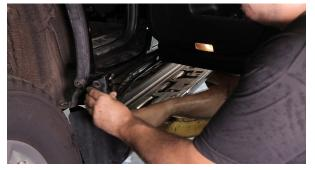
**6.** With the trim on the ground or a workbench, remove the center plastic piece. There are two clips on the front and one on the back. Pry them off with a flat head screwdriver. Then pop it free from all of the plastic tabs all the way down. Finally, pull the front and back of the center piece of the trim. They will be stuck down with double-sided tape.
