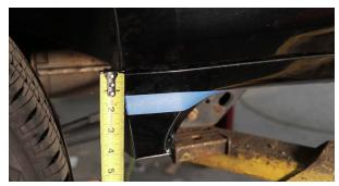
9. Now cut along the line with a cutoff wheel or body saw.
