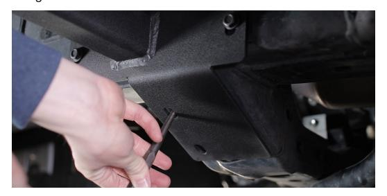
**19.** Once the two holes are drilled, use two 3/8" self-tapping bolts with a 9/16" wrench to secure the bolts. (do not over tighten them, just until they are snug)
