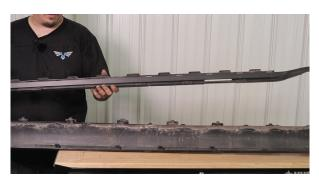
7. Now remove the stock wiring harness from the step. Pop the mounting tabs out of the step with a screwdriver or pry tool, unplug the harness in the center and cut the wiring right at the front and rear lights. We will be reusing the harness to wire in the new LEDs.
