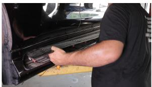
**4.** Remove the three 10mm bolts along the top of the step.
