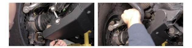
2. Once fully installed, check clearance with your particular wheels by turning full lock in both directions.
