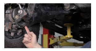
Use the three holes on the lower control arm to mount the skid. Start one side of the skid with a carriage bolt and secure a nut and washer on the top side.
