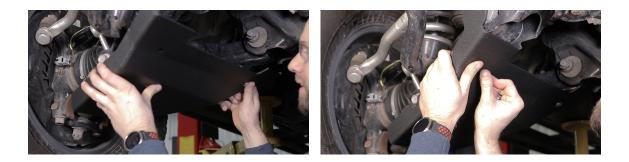
Once you start one bolt, install the other two carriage bolts. The shorter carriage bolt will bolt on closest to the wheel. The 4Runner & Tacoma will use a spacer on the bolt closest to the wheel (between the skid and the LCA). Tighten all of the bolts with a 9/16" end wrench.
