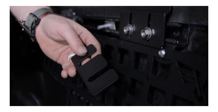
**5.** Install the side bars. Use 2 bolts per side and secure the bolts with a washer and flange nut. There are several mounting options along the uprights.
