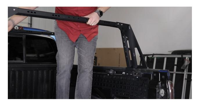
4. OPTIONAL We have provided spacers in the hardare kit. If your uprights do not sit flush on the side of the truck bed then use a spacer. The spacer will install between the upright and the brackets we installed in the side rails.
