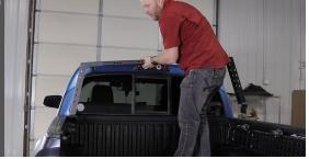
With the rack loosely assembled, bolt it into place. Slide the rack over the studs we installed in step 1 and loosely put a washer and flange nut on each stud. Once you have the rack bolted, push it to the front of the bed.
