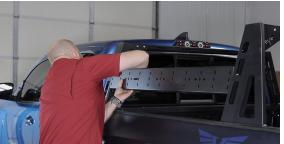
**6.** Install the top bars. Use 2 bolts per side and secure the bolts with a washer and flange nut. There are several mounting options along the crossbars.
