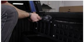
**3.** Assemble the rear rack the same way we assembled the front rack. Make sure the angled portions of the uprights are facing the back.
