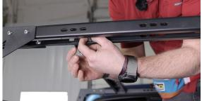
7. Use a 3/16" allen and a 1/2" box end wrench and tighten down all of the bolts. Tighten the top bars first that connect to the crossbars. Be sure to measure the length from the end of the crossbar to the upright. Tighten the side bars next that connect to the uprights. Finally, tighten the carriage bolts once you have centered your rack on the bed of your truck.
