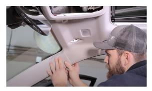
Push the headliner up so the sun visor clips stick out past it and then reinstall the sun visors. The clip will push straight in and the mounting bracket will reinstall using a T-25 torx.
