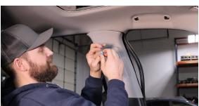
**5.** Next we will move to the rear seats of the vehicle. Remove the grab handles on both sides using the same method as the front handles. Using a pry tool, pop out the dome light (it is held in with clips).
