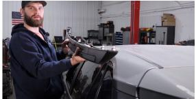
10. Assemble the roof rack on the ground. Start by laying out all of the parts and bolt the crossbars to one side rail at a time using 1/4" button head bolts and washers. We recommend putting a little bit of anti-seize on each bolt. Be sure to install the crossbars with the milled t-nut slots facing up and all to one side.
