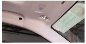
2. Remove the center panel using a pry tool. There are 4 plastic clips holding it in place. After you pull the panel off, disconnect the wire clip.
