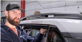
**9.** With the nuts removed, the factory rail will be held in with clips and a small adhesive tape at the front. Pull up to pop the clips and remove the rails.
