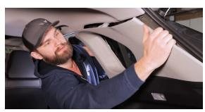
7. Use a panel tool to remove the 3 Christmas tree clips in the rear of the vehicle holding the liner in place.
