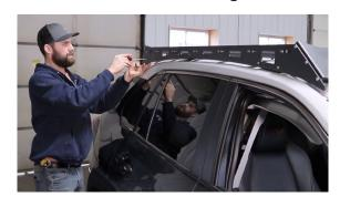
22. We recommend installing some 3M paint protection film under the edge trim on the front and rear fairings. This will protect the paint from any debris that may get caught under the trim over time. Remove the bottom bolt(s) and flip the fairing up out of the way to do so. Then re-install the fairing bolts, slide it down tight to the roof and tighten up the bolts.
