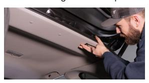
8. At this point the headliner should be dropped down enough to access the roof rail hardware. There will be four nuts per side rail, two in the front above the front grab handles and two above the rear door. Remove them using a 12mm socket or wrench.
