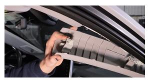
4. Next we will remove the B pillar panel. Start by pull back on the door seal. Pull back on the panel to pop it loose. Remove the clip at the top of the panel so it doesn't poke the liner. Repeat this on both sides.
