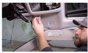
Plug the overhead console back in and snap it back into place.
