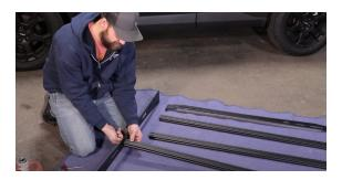
11. Install the front and rear fairings using the same 1/4" bolt and washer with a flange nut on the inside. The front fairing will use 3 bolts per side, the rear will use 2. Slide both fairings up as far as possible and snug them up for now.
