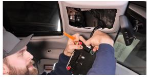
3. Remove the headliner trim around the sunroof by simply pulling it off. Next remove the A pillar panel using a pry tool. You don't need to remove the entire panel, only the top portion of clips need to come out. When you pull the panel off, make sure the clips go back into the clip holder for reinstallation. Repeat this on both sides.
