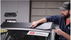
23. Now, reassemble the interior in reverse order of taking it apart. Re-install the rear headliner Christmas tree clips and make sure that the back edge of the headliner sits behind the hatch seal.
