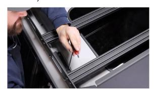
**21.** With the mounts tight to the roof, adjust the height of the rack, ensuring that there is an even gap between the roof and the rack from front to back. With the rack leveled, tighten down the mounting bolts using a 5/32" allen.
