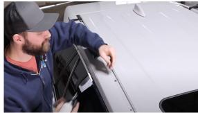
18. Have a friend help you lift the rack onto the roof. Line the mounting holes on the side rails up with the roof mounts. While holding it up, get a bolt through at the front and back to hold it in place.
