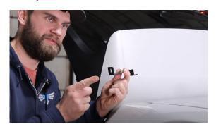
17. Install the provided plastic caps in the remaining 4 clip holes on each side. Put a small bead of RTV around each hole and press them into place.
