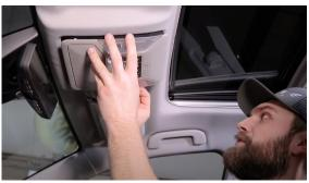
Press the sun roof trim back in place, start in one corner and work your way all the way around.
