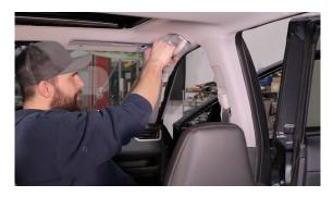
Make sure the A-pillar clips are in place, then snap the A-pillar trim back in place.
