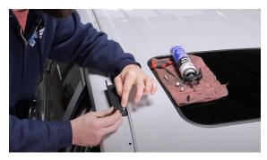
**15.** The middle mounts will have the slight taper towards the front as well as shown. Install them using the same method and hardware as the front mounts.
