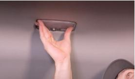
Make sure the headliner is above the door seal and snap the B-pillar trim back in place.
