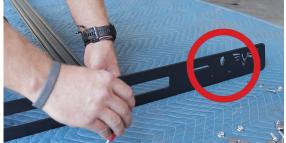
Make sure the t-slot openings are facing up. Center the bars in the slots for now, you will be able to adjust them later.
