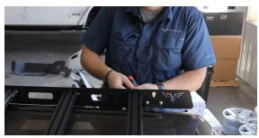
**5.** Go back and tighten down all of the bolts, including the end mount bolts. Reinstall the end caps and you're finished with the installation!
