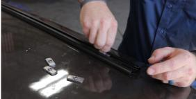
2. Assemble the rack on the ground first. Install all of the bars with the 1/4" hardware (bolts and washers) that we provide except for the rear bar (the mounting location closest to the logo). This will allow you better access to the mounts when you bolt it on the roof.
