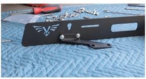
**4.** Mount the rack and center it on the cab. Install the 5/16" button head bolts and a washer to the t-nuts that we installed earlier. Once the rack is mounted you can install the rear crossbar.
