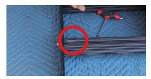
**3.** Install the mounts to the side rails. Make sure the offset is pointed to the center of the rack as shown in the first picture below. Loosely install the mounts so there is room for adjustment when you mount the rack.
