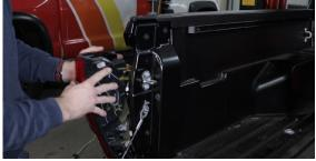
**3.** After you remove the bolt, put the bracket in place. Make sure it sits at a 90 degree angle and is flush with the side of the truck. Mark the bolt holes with a sharpie to determine where to drill.
