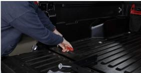
2. Remove the tail light. Use a 10mm socket and remove the bottom bolt along with the second highest bolt. Pull straight back on the tail light once it's loose.
