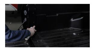
**6.** Put the bracket in place. Loosely install a 7/16" bolt and washer with a flange nut on the other end. For the bottom bolt you will need to reach under the truck and get the bolt started. We are using flange nuts so you will only need to tighten the bolt from one side. Remove the additional hardware on the D ring and reinstall it with a T-30 torx.
