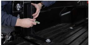
4. Use a small drill bit and begin drilling the holes that you marked in step 3. Once you have the holes drilled, use a step bit to make the holes bigger. We are using 7/16" hardware so you will need to drill up to 7/16".
