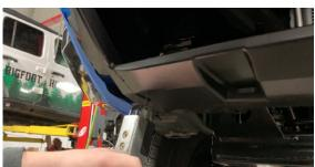
**3.** After you remove the valance, remove the splash guard.
