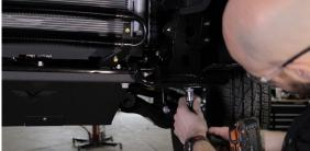
7. Before we can install the bumper we need to move the cooler back. Start by removing the 12mm bolt on both sides of the cooler.
