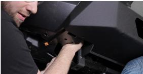
Using a 3/4" socket, install a 1/2" bolt that we provide on the bottom bracket of the bumper. Secure this bolt with a washer and flange nut.
