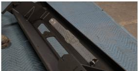
2. Remove the eleven 10mm bolts along the valance, then use a pry tool to pop the front plastic panel off. Once you remove the panel, you can cut the very small lower valance off. (This will be hidden by the plastic panel if you ever need to go back to stock)
