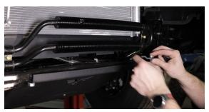
Install the other 2 brackets in the front using a 5/16" button head bolt and the stock bolts we removed earlier. Make sure the brackets are pointed straight back toward the truck.
