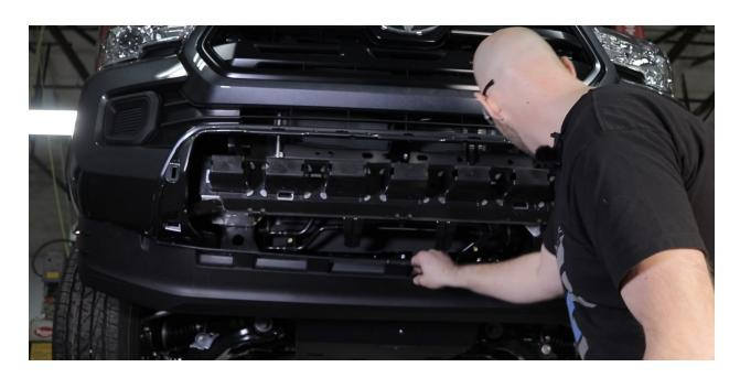
4. Next we will remove the crash bar. There is a plastic cover over the crash bar that we will remove by pressing on the clips. Use a 14mm socket to move the 6 nuts holding the crash bar in place. Remove outer trim screws from the bottom of the plastic valance and remove crash bar assembly. You may need to drill out the rivets holding the reinforcement brackets to the crash bar to remove it.
