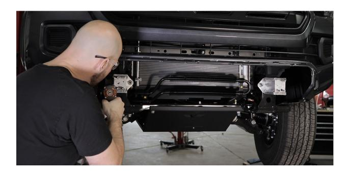
**6.** Using a 14mm socket, remove the 4 bolts holding in the side blocks as shown in the picture below. There is 1 bolt on the drivers side and 3 on the passenger side. The blocks will slide out of the frame.
