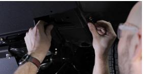
After you secure the inner fender, use a 5/16" drill bit and drill a hole in the plastic that covers the pre-drilled hole in our bumper. Use a 3/16" allen to tighten the 5/16" bolt with a flange nut.
