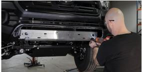
**5.** Remove the aluminium stand off blocks from the crash bar with a 14mm socket.
