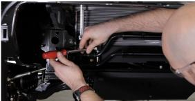
Remove the flap under the passenger side to reach the last 12mm bolt. Install the small bracket we supply with a 5/16" button head bolt. Use the stock bolt to secure the bracket to the frame.
