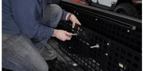
3. Next we will install the lower mounts that secure the panel to the truck.
