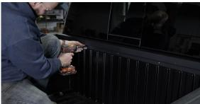
**5.** Use the 90 degree brackets we provide and reinstall the bolts. Hold the bracket straight while you tighten them.
