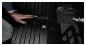
**4.** Using a T-30 torx, remove the three bolts along the top of the bed.
