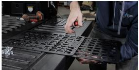
2. We will be installing a high lift jack on our panel. Insert the two carriage bolts through the holes located on the center panel. Loosely install these bolts so you can adjust them later.
