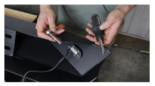
**3.** Bolt on the logo accent plates using a button head stainless bolt and a flange nut (3 bolts per plate).
