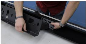
2. Install the LED lights using the provided button head bolts, washers, and lock nuts. Make sure the lights are centered in the hole and tighten them down using a 3mm allen and a 5/16" socket or wrench
