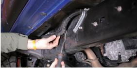
**6.** Use a pry tool to remove the plastic cap and the black sticker.
