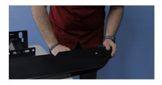
4. Install the rest of the button head bolts to mount the legs to the slider. Leave the bolts loose so you can move the slider back and forth to align it on the truck once its mounted. From this point on, they will mount to the truck in the same way as our Strike Rock Sliders
