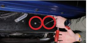
**8.** Use a jack to lift the slider into place. Make sure the wire harness is out of the way before bolting the slider to the frame.
