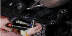
13. Reconnect the brake line brackets and the electric box. Go back and tighten down all of the bolts then you will be finished with the install.
