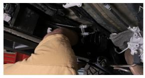
**12.** Next, use a magnet to insert the 1/2" nut through the frame hole. Then thread the 1/2" bolt through the bottom hole and into the nut. Use a 3/4" socket to tighten it down.
