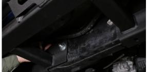
**9.** With the slider jacked into place, replace the bolt that we removed earlier with the bolt that we supply in the same crossmember. Loosely install this bolt.
