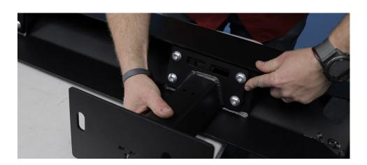
**5.** Remove the bolt that connects the crossmember to the frame rail. Use a 14mm socket to remove the bolt. Use a pry tool to move the wire harness out of the way.
