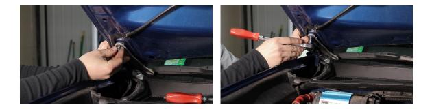
**3.** After you get the mount installed, push up on the bottom of the bracket to push the threads through the hole. Install the small rubber washer with the brass nut on top. You can use channellocks to tighten the brass nut but make sure you don't overtighten.
