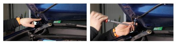
**2.** Line the bracket up with the hinge. Make sure your hinge is lined up with the marks we made with a sharpie. Using a 12mm socket, reinstall the two factory bolts to secure the bracket to the hood.
