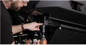
Use a 14mm socket and tighten the rest of the nuts holding the bumper in place.
