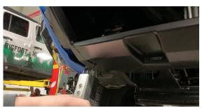
**3.** After you remove the valance, remove the splash guard.
