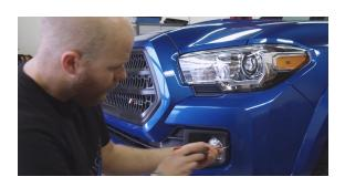
2. Next we will cut a straight line from the factory fog light mount to the edge of the factory bumper. We used a laser level to get the most accurate straight line. Use a tape measure and measure from the ground to the straight line and veryify that the line is level (only measure from the ground if the ground is level. You want to make sure your reference point is level before making the cut).
