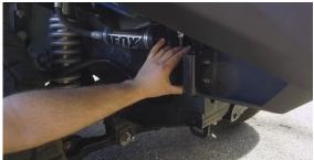
16. Push the large bolt that we provide through the reinforcement bracket and loosely install it with a washer and a nut. Make sure you don't overtighten the large bolt that we provide. Reinstall the outer nuts.
