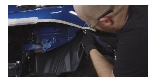
**9.** Next we will trim the inner fender liner. Using a sharpie, mark a line that is flush with the support bracket right above the inner fender liner. Use a utility knife to trim the line.
