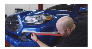
**4.** With your choice of cutting tool, carefully cut on the line we made. We will be using a 4" cut off wheel to get an accurate cut. We used a smaller body saw in the bottom right image so we didn't cut into the inner fender liner.
