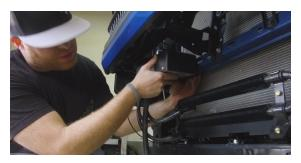
**14.** Have a friend help you lift the bumper onto the truck. Tighten the outer bolts using the factory nuts with a 14mm wrench. There will be 4 bolts on each side.
