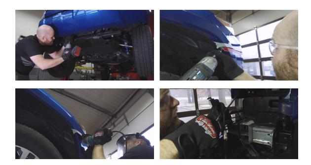
**6.** After you remove the factory bumper, remove the plastic cover from the crash bar.
