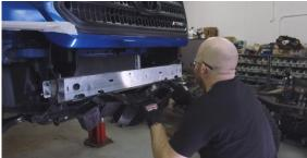
7. Using a 14mm socket, remove the 6 nuts holding the crash bar in place.
