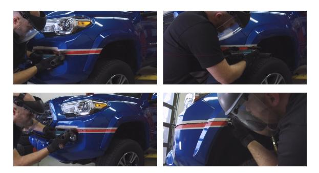
**5.** Remove the bottom bolts holding the factory bumper in place using a 10mm socket. Remove the 10mm bolts on the side as well as the clips to remove the bumper. You will need to disconnect the fog lights using a pry tool.
