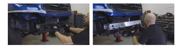
**7.** Using a 14mm socket, remove the 6 nuts holding the crash bar in place. Next remove the 6 nuts hold the 2 crash bar brackets in place.
