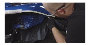
**9.** Next we will trim the inner fender liner. Using a sharpie, mark a line that is flush with the support bracket right above the inner fender liner. Use a utility knife to trim the line.
