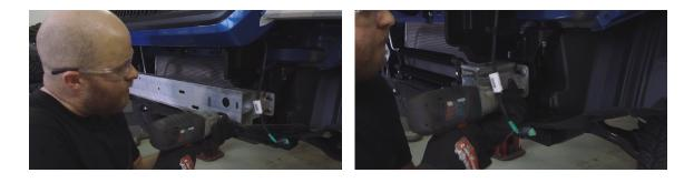
**8.** Go back and remove any plastic brackets that are below the line we cut. You can now remove the tape and lightly sand the line to make it smooth.
