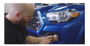
2. Next we will cut a straight line from the factory fog light mount to the edge of the factory bumper. We used a laser level to get the most accurate straight line. Use a tape measure and measure from the ground to the straight line and veryify that the line is level (only measure from the ground if the ground is level. You want to make sure your reference point is level before making the cut).
