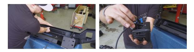
**12.** Next we will install the winch. There are four holes on the base of the bumper where you can mount your winch and access holes on the bottom of the bumper to secure the winch to the bumper.
