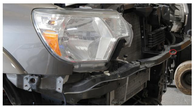
19. The two 90° brackets will bolt on the underside of the Strike bumper using a button head bolt and flange nut. The plastic piece under each headlight will then snap back into them.
