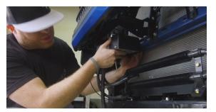
**14.** Have a friend help you lift the bumper onto the truck. Tighten the outer bolts using the factory nuts with a 14mm wrench. There will be 4 bolts on each side.
