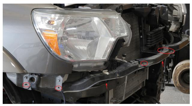
**18.** The new Victory valance piece will attach to the front, center stud using the stock nut(circled below).
