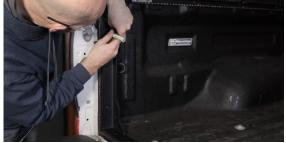
**3.** Use a small drill bit and begin drilling the holes that we marked in step 2. Once you have the holes drilled, use a step bit to make the holes bigger. We are using 7/16" hardware so you will need to drill up to 7/16".
