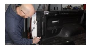
**5.** Using a T-30 torx bit, remove the two bolts holding the brake light in place. Once the brake light is loose, pull it away from the truck then pull straight back.
