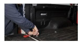
2. After you remove the bolt, put the bracket in place. Make sure it sits at a 90 degree angle and is flush with the side of the truck. Mark the bolt holes with a sharpie to determine where we will drill.
