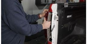
**6.** After you remove the brake light, put the bracket in place. Loosely install a 7/16" bolt and washer with a flange nut on the other end. For the bottom bolt you will need to reach under the truck and get the bolt started. We are using flange nuts so you will only need to tighten the bolt from one side.
